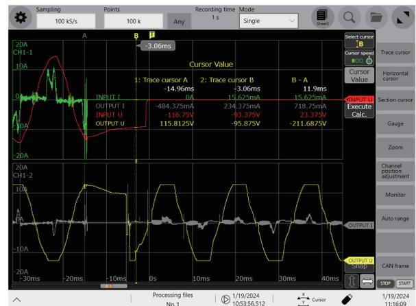
Example waveforms of primary and secondary voltages during UPS operation
