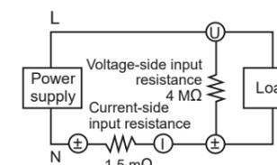
Power including loss is measured by means of the voltage input terminal's input resistance.
