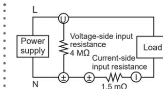
Power including loss is measured by means of the current input terminal's input resistance.
