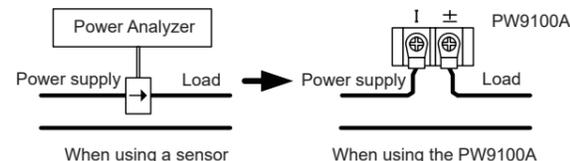
To ensure accurate measurement, do not connect output cables and measurement cables in parallel.
