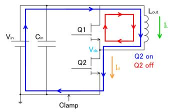
E.g. double pulse test for GaN device.
