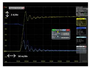
CH1 (yellow): Id, turn on current CH4 (blue): Vds, turn on voltage Math1 (cyan): Switching loss, CH1 x CH4
