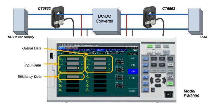
Setting example of wire connection or display position using Models PW3390 and CT6863 (200A rated) x 2
