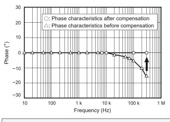
Phase compensation of current sensor with memory When the current sensor with memory is used, the phase of the current sensor is automatically corrected.
