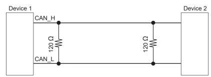
• If the terminator is set to ON, the 120  $\Omega$  resistors are inserted between the differential signals of the CAN bus inside the LR8102.
