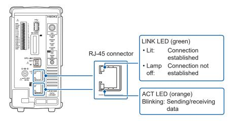
The LINK LED lights up when the instrument is properly connected to the network and available. If the LED does not light up, the instrument or connected devices may have a problem or the LAN cable may be broken.
