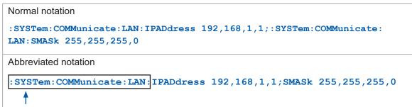
This part defines a current path, which can be omitted in the subsequent commands.
