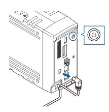
Turn OFF the instrument and remove the AC adapter.
