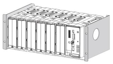
**3** Secure the instrument with the bracket with screws at the back.
