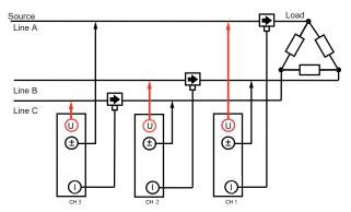
Normal connections when using the PW9100A
