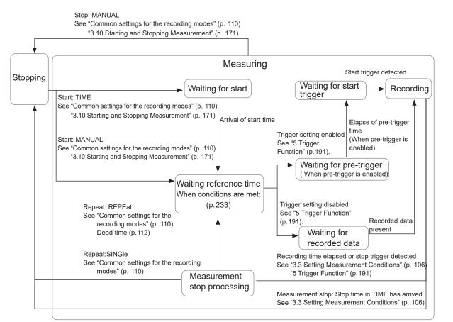
When simple measurement is performed using the ": STARt: PWCHeck" command
