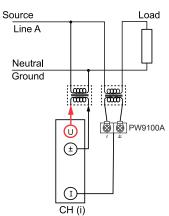
2 Connection (Preparation for Measurements)
