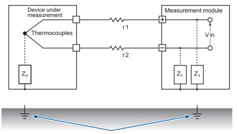
Temperature measurement using a thermocouple is affected by noise unless both the instrument to be measured and the measurement module are connected to the ground. Be sure to ground the AC adapter when using it.
