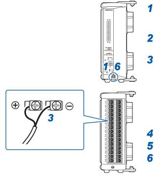
Remove the screw for the terminal block cover.
