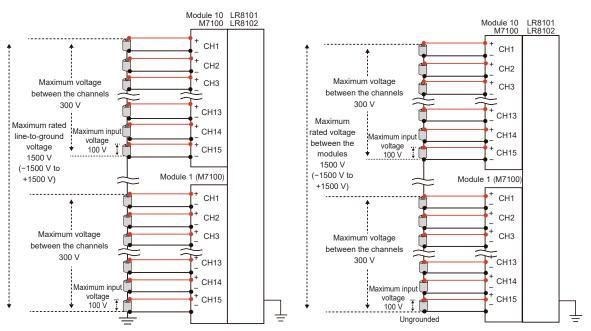
If you use modules with differing maximum rated voltages between modules for a measurement target connected in series, such as a battery pack, the specifications of the module with the lower maximum rated voltage between modules will apply.
