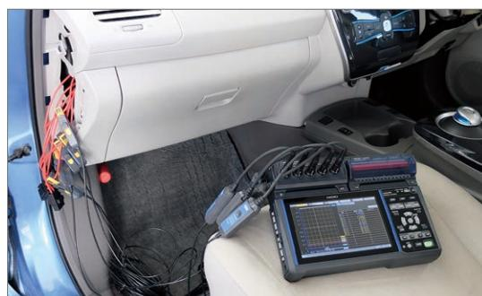
The LR8450 and AC/DC Current Sensors CT7812/CT7822 are ideal for measurements made in EV power management for the following three reasons:
