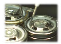
The probing repeatability is extremely important for measuring ultra-low resistance with high-accuracy. Excellent probing precision and repeatability accuracy keeps exactly same measurement point, ensuring high stability measurement. Keeps stable 4-terminal measurement method even though extreme narrow space like external case edge of negative electrode of cylinder-shape cell.
