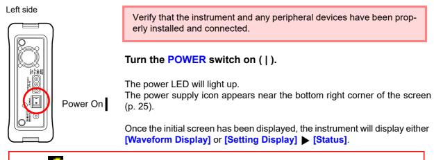
If the " ... indicator is not displayed, the instrument is not being powered from the AC line. In this state, the battery charge will be depleted if measuring for a long time, and measurement may be interrupted. Verify that the AC adapter is securely connected to an AC power source and to the instrument.
