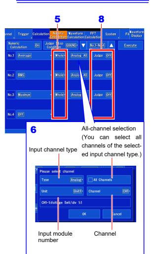
NOTE If measurement is disabled for a channel selected as a calculation target channel, the calculation will not be performed. Depending on the calculation type and input channel type, you may not be able to select all channels.
