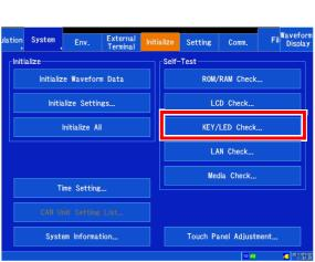
If any key malfunctions or is not recognized, you will be unable to end the key check. If this occurs, you can return to the original screen by pressing the START key and the STOP key at the same time. The instrument may be experiencing an error or malfunction and should be repaired.
