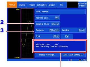
The recording time and maximum recording time will be displayed based on the timeaxis and recording length settings.
