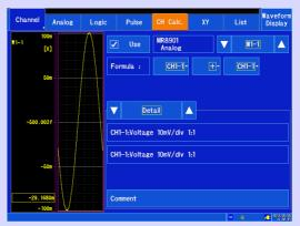
**Inter-channel calculation channel settings** Use when measuring waveforms calculated between analog channels.
