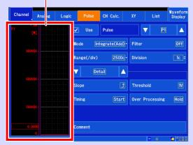
**Pulse channel settings** Use when making pulse (integration, rotational speed) measurements.
