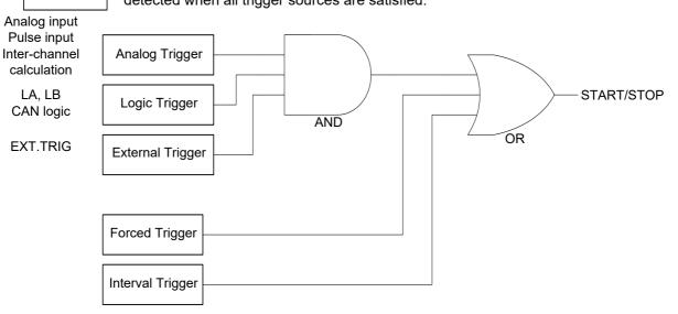
**NOTE** Forced triggers and interval triggers cannot be set as stop triggers.
