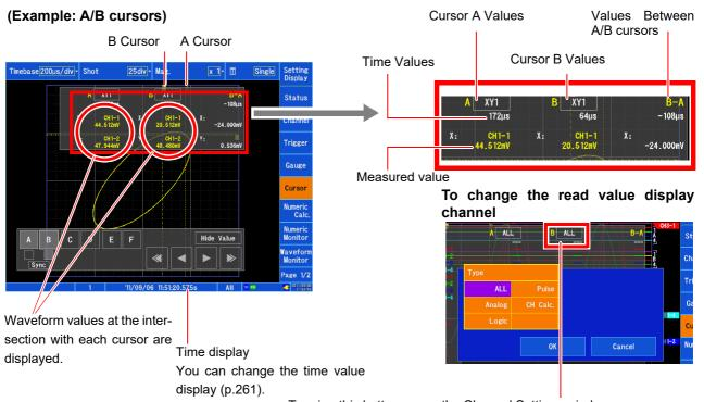
Tapping this button opens the Channel Settings window. You can select the channel for which you wish to display cursor read values.
