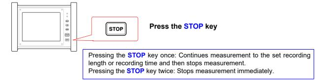
**NOTE** If you stop measurement by pressing the **STOP** key twice, the last data point may not be recorded.
