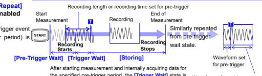
After starting measurement and internally acquiring data for the specified pre-trigger period, the [Trigger Wait] state is activated. Wavefc
