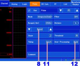
When **[Hold]** is selected and the set channel is the trigger source, the trigger will not be applied while the trigger level is exceeded during the pre-trigger wait period. If the trigger is not applied, check the integrated value on the waveform monitor.
