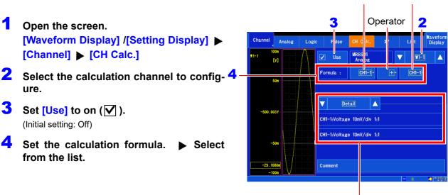
You can check the settings of the analog channels that have been allocated to the calculation formula by selecting [Detail].
