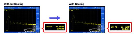
Setting example: To display measurement data on this instrument so that it corresponds to that on a sound level meter.
