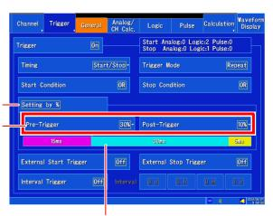
You can check how the set pre-trigger or post-trigger time compares to the total recording time on the [Setting Display]u[Trigger]u[General] screen.
