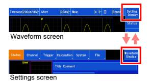
You can switch between the Waveform screen and the Settings screen by tapping the tab on the right side of the screen.
