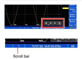
On screens that support scrolling (screens on which the Arrow window is shown), you can scroll waveforms by tapping in the direction in which you wish to scroll. See: "Scrolling waveforms" (p. 118)
