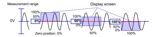
The setting range varies with the vertical axis magnification/compression rate setting. The maximum setting range 100 yields values ranging from -10,000% to 10,100%.
