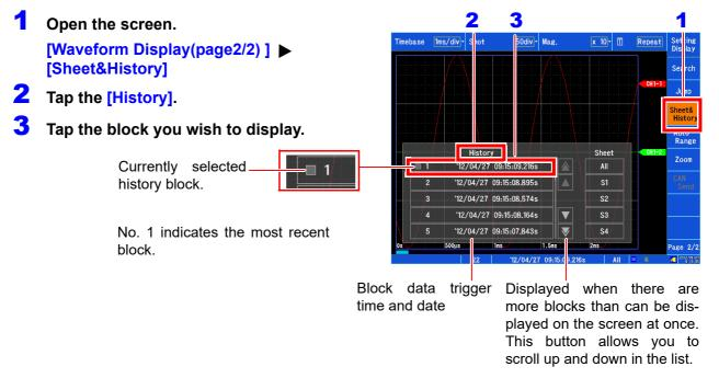
You can also check up to 200 events of the past trigger times (when the trigger is not used, the measurement start time).
