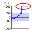
When broken wire detection is enabled, readings that exceed the range's measurable range by a large margin will be treated as indicating a broken wire.
