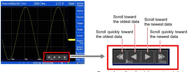
The waveform will scroll each time you tap a button. Strong taps\* cause the waveform to scroll quickly, and continuing to touch a button causes the waveform to scroll continuously.
