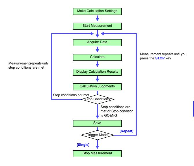
**NOTE** Auto saving is not performed until the stop condition is met after calculation judgment.
