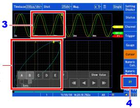
**NOTE** When performing compositing on the [Waveform+XY] screen, the compositing range will not change until you tap [XY].
