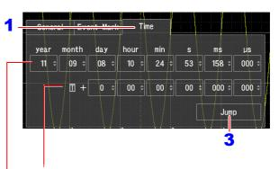
Time from a trigger (relative time) T+: After the trigger; T-: Before the trigger
