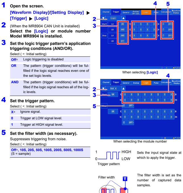
Number of samples: 1 div = 100 samples (when the display magnification is set to 1).
