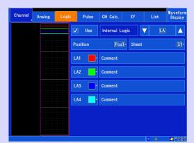
Logic channel settings Use when making logic measurements. See: "Configuring logic channels" (p. 71)
