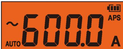
The warning backlight works only for the present measured value. The warning backlight does not work for the freezing value and recorded values of the MAX, MIN, AVG, PEAK MAX, and PEAK MIN display functions.
