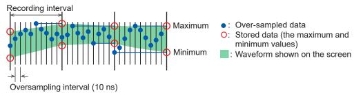
A set of sampled data acquired using the envelope consists of two values: the maximum value and the minimum value. These values are taken from the measured values acquired by sampling an input signal at an over-sampling rate during the recording interval chosen in the [Sampling] box. The screen displays a vertically wide waveform line. When saved in an external storage device, the data set that consists of the maximum and minimum values is stored for a single instance of measurement.
