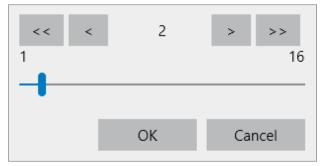
Use the arrow keys, two-headed arrow keys, and slider to select a block number, and tap **[OK]** to display instantaneous waveforms contained in the selected-numbered block.
