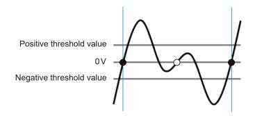
After a zero-cross point is detected (• mark), points at which 0 V is crossed (O mark) will not be treated as the next zero-cross point unless the signal has exceeded the hysteresis width (the range between the positive hysteresis threshold value and the negative hysteresis threshold value).
