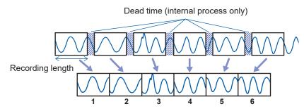
The instrument records a recording length of waveform data once per block.
