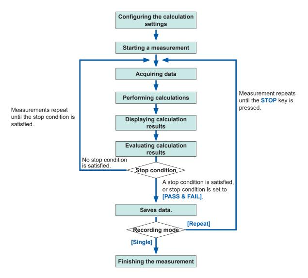
Automatic saving is not carried out until the stop condition is satisfied at the end of calculation evaluation.
