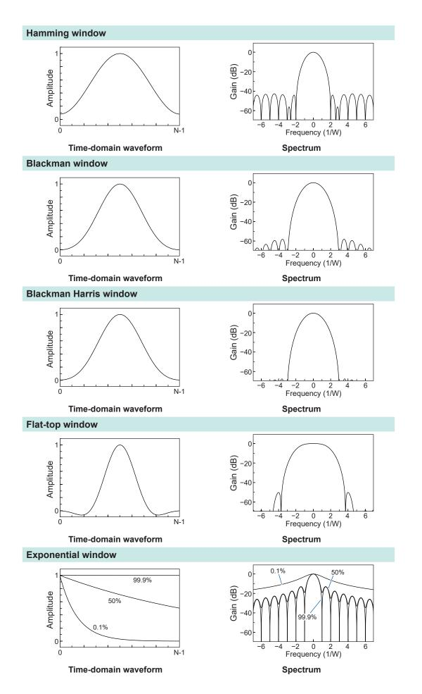
The following example shows the analyses of input sine waves, which has a frequency of 1050 Hz and 1150 Hz, with different window functions.
