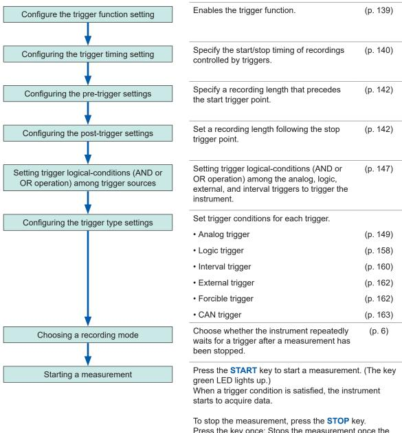
Press the key once: Stops the measurement once the instrument has acquired the specified recording length of data.
