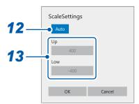
**12** Tap the [Scale Settings] button to set the scale setting of calculation results to [Auto] or [Manual].
