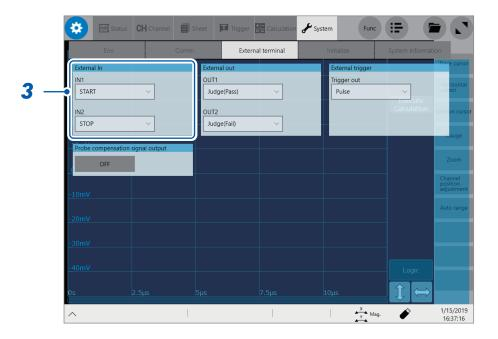
**3** Tap the [IN1] and [IN2] boxes in the [External In] area in turn, and then from the list, choose an action performed when an input signal is inputted.
