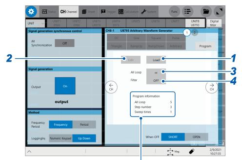
Displays the looping count, step number, and sweeping count of the still-in-progress process. When you have set the whole looping times to infinity, the instrument will show [∞] as the entire looping count of the still-in-progress process repeating more than 50,000 times.
