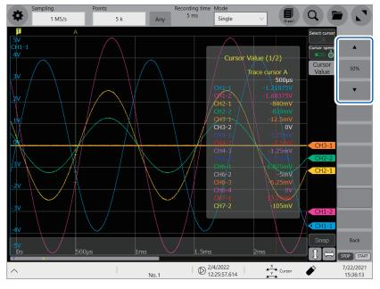
Tapping [▲] or [▼] allows you to change the opacity of the screen background between 0% and 100% in 10 percent points increments.
