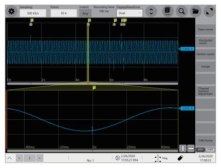
The trend waveforms (on the upper screen) have the trigger marks  $\mathbf{I}$  and block numbers that indicate the positions of the instantaneous waveforms.
