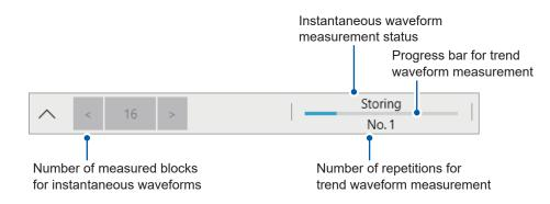
4 (When the displayed waveforms are set to [Dual] or [Instantaneous])
