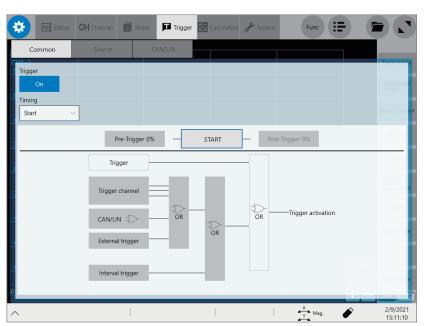
The instrument can record instantaneous waveforms using triggers under certain conditions only. See "5 Configuring the Trigger Settings" (p. 137).
