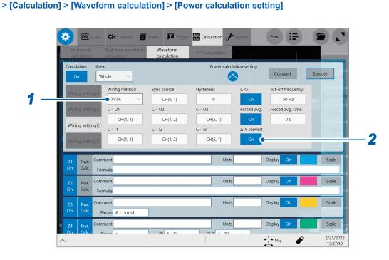
**1** Tap the [Wiring method] box and select [3V3A].
