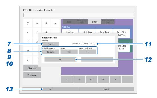
7 Tap the [Channel] box, and then choose a calculation target channel from the list (choose "UNIT1-CH1" of built-in modules).
