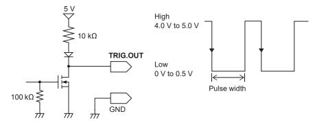
When the auto-range function is used, the instrument is triggered, outputting the TRIG.OUT signal. Be careful when performing auto-range measurement while using the TRIG.OUT signals.
