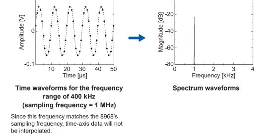
To prevent the imaging phenomenon when analyzing waveforms using the FFT function, be sure to check the unit's maximum sampling frequency prior to measurement.
