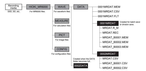
When dual-sampling waveforms are collectively saved or divided before saved into display blocks, the instrument newly creates the folder with the name of the waveform file name preceded by a running number and saves all the files in the folder.
