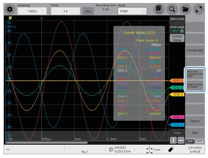
Tapping [Show only channels in the sheet] can only display channels in the present sheet. Tapping [Select channel to display] allows you to select channels of which you want to display cursor values.
