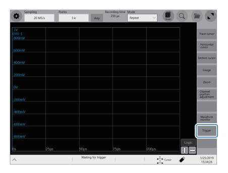
Tapping **[Trigger]** on the right side of the waveform screen allows you to manually trigger the instrument while the instrument is waiting for a trigger.
