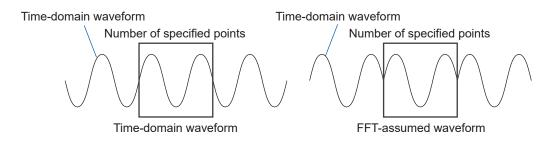
When the number of FFT calculation points is equal to an integer multiple of the input signal frequency, a single line spectrum is obtained. However, if the number is unequal to an integer multiple of the frequency (with the result that the FFT-assumed waveform has discontinuous points), spectral lines spread, resulting in failure of production of a line spectrum. This phenomenon is called the leakage error (as shown below).
