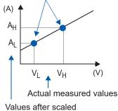
When changing the value with the **[Ratio]** setting, the instrument does not change the values for  $V_L$  or  $V_H$ , but the values for  $A_L$  and  $A_H$ , all of which have been specified with **[Method]** set to **[2-Point]**.
