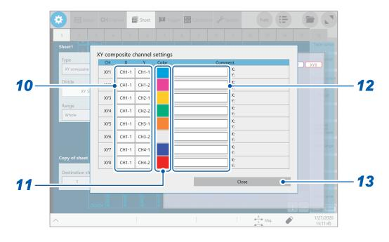
**10** Tap a channel number button, and then from the list, choose channels to be assigned to the X and Y axes of the XY channel you chose.
