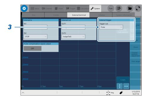
**3** In the [External trigger] area, tap the [Trigger out] box, and then from the list, choose a signal output method (the signal is outputted through the trigger output terminal).
