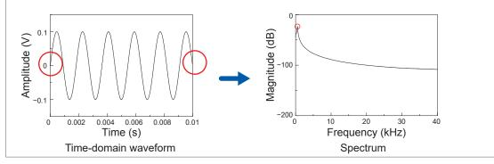
The window function has been created to suppress such leakage errors. The window function smoothly connects each cropped end of a time-domain waveform.
