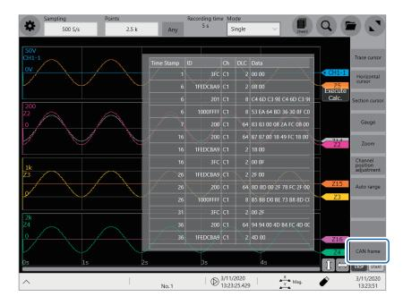
The monitor table can be displayed on the waveform screen.
