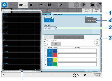
The instrument displays the waveform screen when a logic channel is chosen. You can check display positions of the logic signals.
