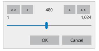
**3** Select a block number using the arrow keys ([<] and [>]), the double-arrow keys ([<<] and [>>]), or the slider and tap [OK].
