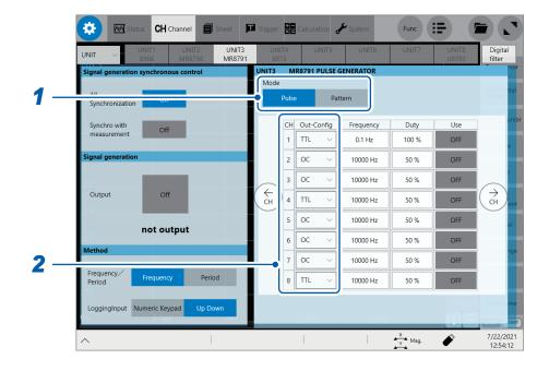
**1** Tap the [Mode] button and select the output waveform type.
