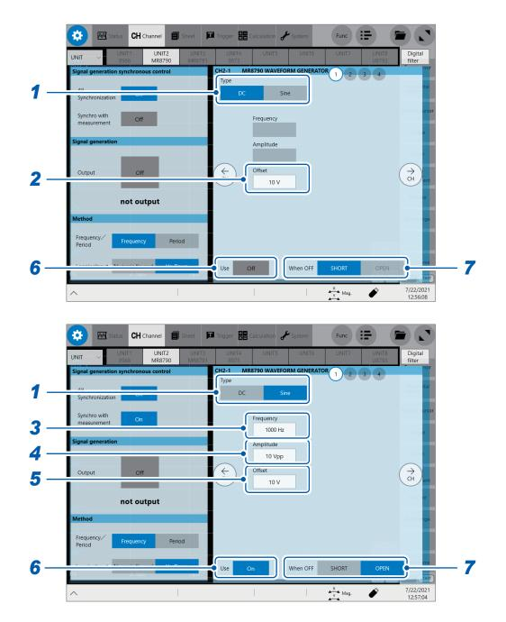
**1** Tap the [Type] button and select the waveform type.
