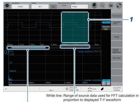
Bar indicating the range being displayed in proportion to whole acquired data Gray bar: T-Y waveform position
