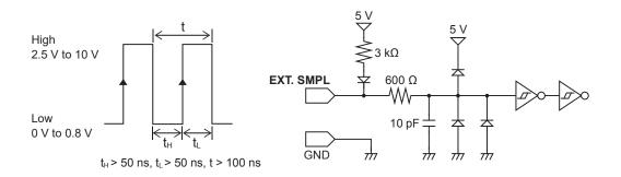
• If a sampling signal with 5 MHz or more is inputted, trigger points are delayed by one sample.
