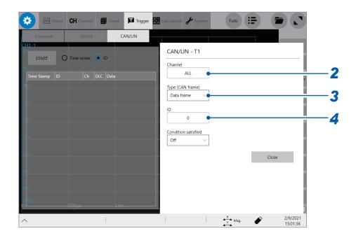
**2** Tap the [Channel] box, and then from the list, choose a channel of which you wish to configure trigger conditions.
