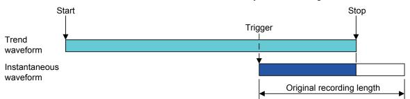
For repetitive measurements, the instrument clears waveforms every time it finishes recording of trend waveforms, and then restarts recording waveforms from the beginning. At this time, instantaneous waveforms are also recorded from the start block. You can stop recording by pressing the STOP key
