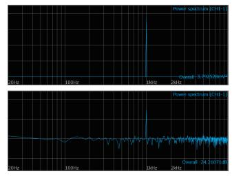
**Normal display** Horizontal axis: logarithmic Vertical axis: amplitude (linear)
