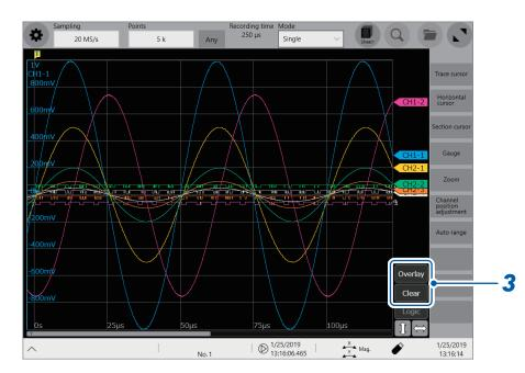
**3** Overlay the waveforms manually (leaving any waveforms to be displayed on the screen). Tap the button on the right side of the waveform screen.
