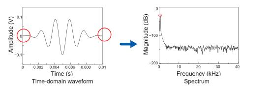
The following figure illustrate the time-domain waveform multiplied by the window function and its spectrum.
