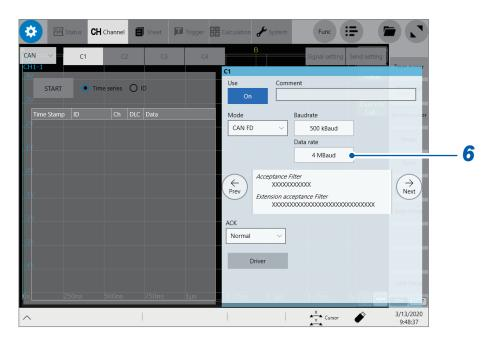
Tap the [Data rate] box, and then from the list, choose a baud rate used in the data phase.
