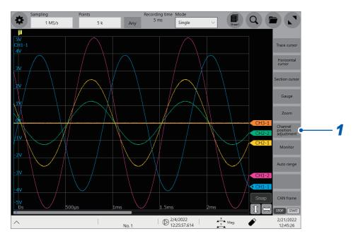
The channel position adjustment screen is displayed.
