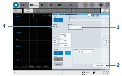
Current sensors to be connected determine whether the instrument automatically recognizes mode or whether you have to choose a current sensor setting.
