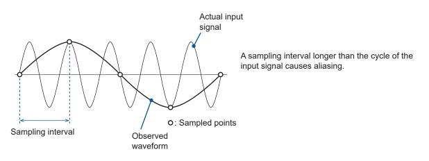
To plot a sign wave that allows you to observe the peaks without any aliasing, the instrument needs to sample the waveform at a minimum of 25 points per cycle.
