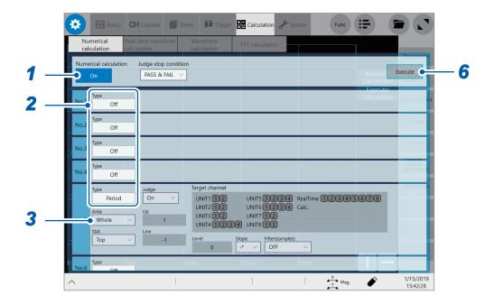
**1** Tap the [Numerical calculation] button to set it to [On].
