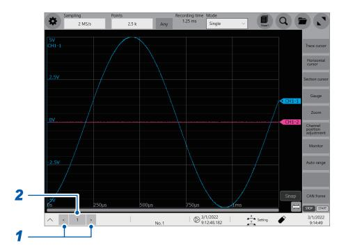
**1** Tap the [<] and [>] keys to cycle through the block number shown on the waveform screen.
