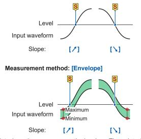
The point where the max. crosses the level The point where the min. crosses the level
