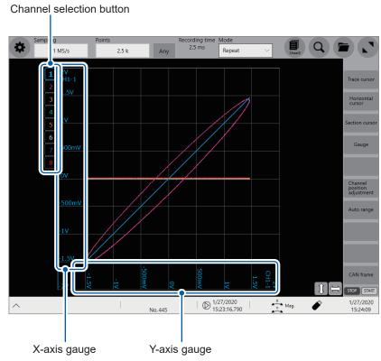
The X-axis and Y-axis gauges indicate the values of channels of each axis assigned to the chosen composite channel.
