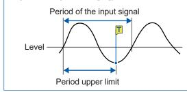
The period-trigger condition is satisfied when the upper limit of periods elapses before a rising slope of an input signal crosses the reference voltage level.
