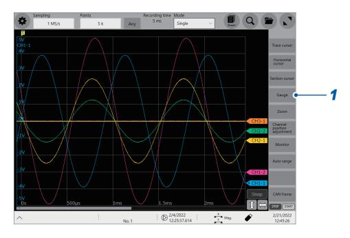
**2** Choose gauges to be displayed from among [Gauge A] through [Gauge H]. The screen display the gauges at the left.
