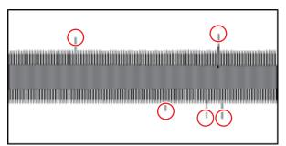
By observing trend waveforms, you can roughly check variation of waveforms under measurement. Instantaneous waveforms can be captured by configuring trigger settings, allowing you to examine abnormal phenomena (circled) closely.
