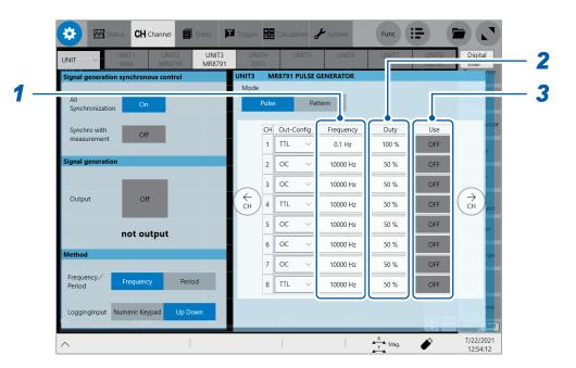
**1** Tap the [Frequency] box and enter the frequency (in 0.1 Hz increments).
