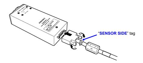
**3** Connect the other end of the cable to the main unit's sensor unit connection port and tighten the connector securely in place with the mating screws.
