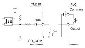
PLC Output (Source Output) Connections
