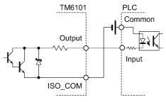
PLC Input (Source Input) Connections
