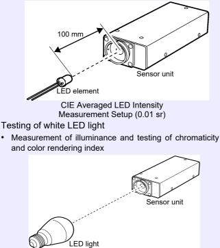
Measurement of total luminous flux, chromaticity, and color rendering index
