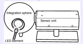
Total Luminous Intensity Measurement Setup
