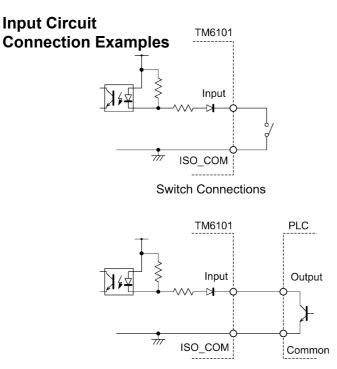
PLC Output (Sink Output) Connections
