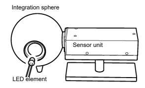
Total Luminous Flux Measurement Setup
