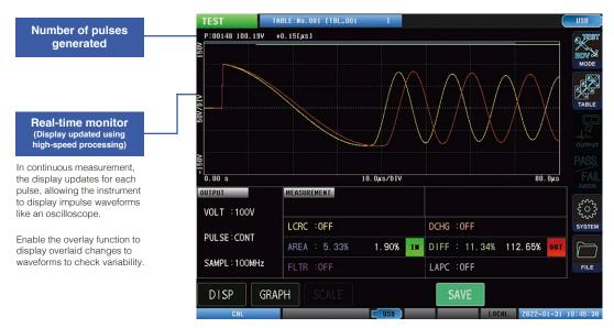
During continuous measurement, only measurement data for the most recent pulse is maintained by the ST4030A.
