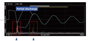
High-frequency discharge components are isolated by a proprietary Hioki filtering process.
