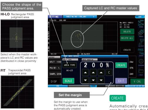
Select when the motor's rotor has been attached and the distribution of the LC and BC values assumes a belt shape according to the rotor position or angle
