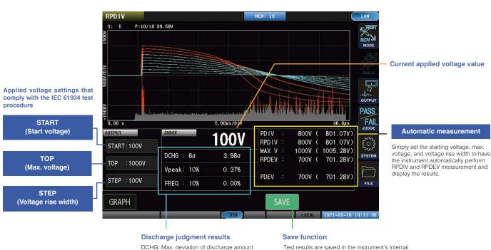
Vpeak: Max. misalignment width from the standard peak voltage value FREQ: Max. misalignment value from
