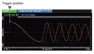
Make judgments based on the response waveform using the rising edge of the application waveform as the trigger (the same approach used by conventional testers).
