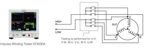
Automate testing using a setup such as the one shown below by using a High Voltage Scanner 3930 to switch the measurement circuit.
