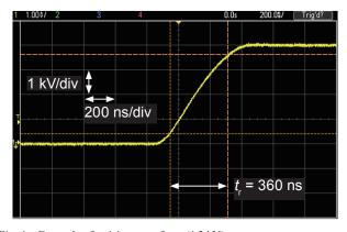
Fig. 4. Example of a rising waveform (4.2 kV).
