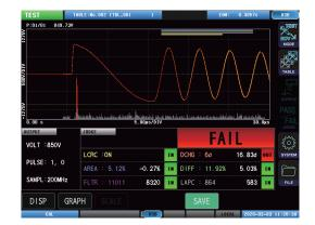
Fig. 7. Waveform graph display screen (with discharge).
