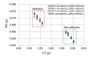
Fig. 14. Differences in LC and RC values caused by applied voltage.
