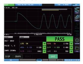
Fig. 8. Waveform graph display screen (without discharge).
