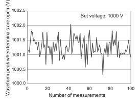
Fig. 6. Variability in impulse waveform peak values.
