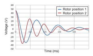
Fig. 12. Voltage waveform variation when rotor is rotated.
