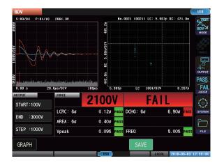
Fig. 9. BDV test screen.
