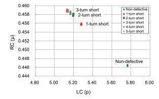
Fig. 15. Distribution of LC and RC values for a non-defective coil and coils with shorts involving various numbers of turns.
