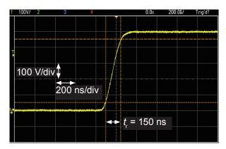
Fig. 3. Example of a rising waveform (500 V).
