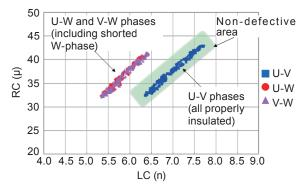
Fig. 13. Distribution of LC and RC values between each phase of a motor whose W-phase is shorted.
