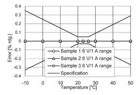
Fig. 17. Active power temperature characteristics: DC (0% f.s.).
