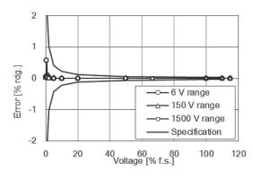
Fig. 4. Voltage linearity: AC+DC.
