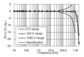
Fig. 9. Voltage frequency characteristics: AC+DC.
