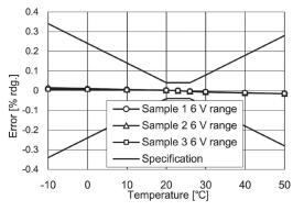
Fig. 14. Voltage temperature characteristics: AC+DC (100% f.s.).
