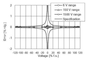
Fig. 3. Voltage linearity: DC.
