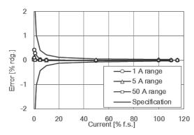
Fig. 6. Current linearity: AC+DC.
