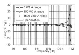
Fig. 11. Active power frequency characteristics: AC+DC.
