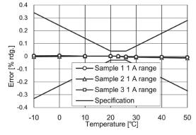
Fig. 16. Current temperature characteristics: AC+DC (100% f.s.).
