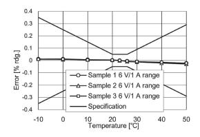
Fig. 18. Active power temperature characteristics: AC+DC (100% f.s.).
