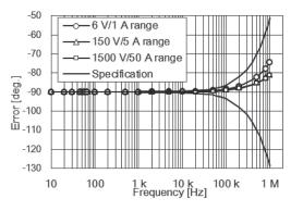
Fig. 12. Phase frequency characteristics: AC+DC
