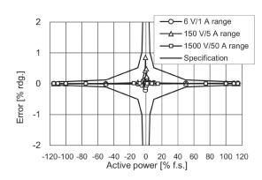
Fig. 7. Active power linearity: DC.
