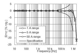
Fig. 10. Current frequency characteristics: AC+DC.
