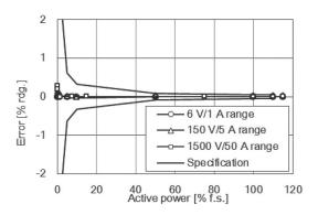
Fig. 8. Active power linearity: AC+DC.
