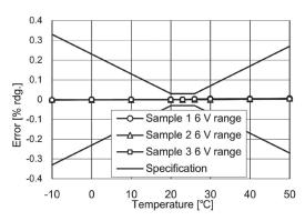
Fig. 13. Voltage temperature characteristics: DC (0% f.s.).
