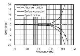
Fig. 2. CT6862 phase characteristics correction.
