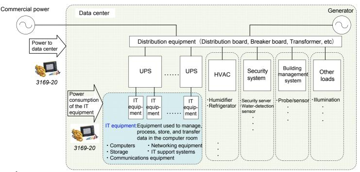
1. Measure the power consumption (W) of all equipment in the data center and the power consumption (W) of the IT equipment.
