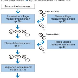
Return to the line-to-line voltage measurement screen.
