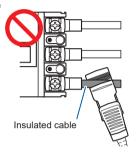
The insulated cable is inserted too close to the pivot point.
