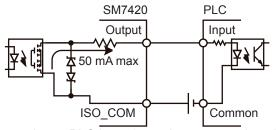
Connection to PLC input (negative common input)
