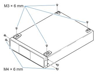
1 Remove the stands from the bottom of the instrument, and the screws from the sides (4 near the front).
