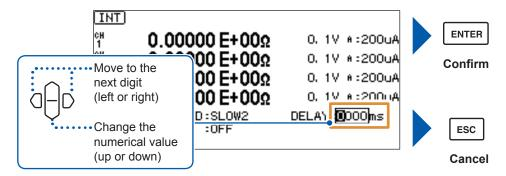
The numerical value can also be changed with the numeric keypad. See "Methods for changing numerical values" (p. 25).
