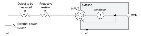
When using the external power supply, insert a protective resistor so that a current flowing through the instrument is reduced to the rated current or less even if the terminals of the object to be measured are short-circuited with each other.
