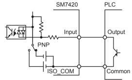
Connection to PLC output (PNP output)
