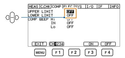
2 If the upper limit and lower limit settings are set to [ON], set the numerical value.
