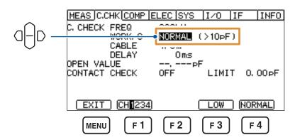
If the capacitance of the object to be measured is unknown, select **[NORMAL]** and then execute the open correction with the object connected to the instrument to obtain its capacitance. Select whether **[LOW]** or **[NORMAL]** depending on this measured capacitance. See "4.6 Canceling Capacitance of Measurement Fixture (Fixture Capacitance Open Correction Function)" (p. 52).
