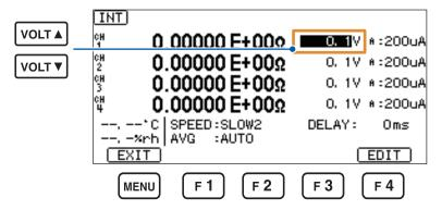
**3** Press the SPEED key to set the measurement speed to [SLOW2]. (p. 36)
