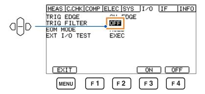
2 If [ON] is selected, set the response time (time during which the TRIG signal remains in the on state).
