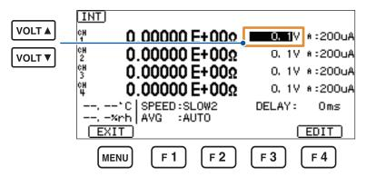
Pressing the F4 key [EDIT] enables the numerical value to be changed in increments of 0.1 V.
