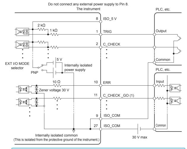
Share the ISO\_COM for the common terminals of the input and the output signals.
