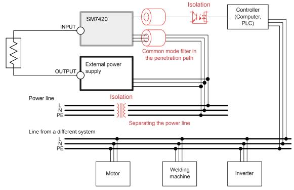
Figure 6 Conductive Noise Countermeasures
