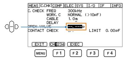
The open correction is executed, acquiring the correction value.
