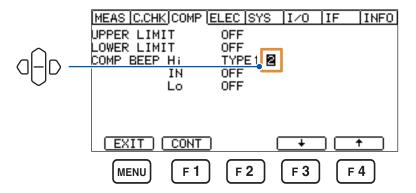
Press the F3 key [ $\downarrow$ ] or F4 key [ $\uparrow$ ] to change the number of times. Press the F1 key [CONT] to use the continuous sound setting.
