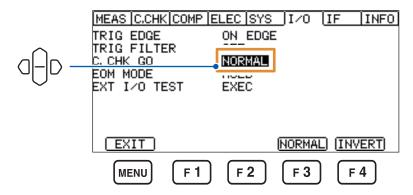
When the contact check is disabled, the instrument always gives fail judgments and thus outputs the Off signal.
