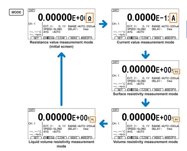
Measurement conditions must be set to measure surface resistivity and volume resistivity. See "4.8 Setting Resistivity Calculation (Resistivity Measurement Function)" (p. 55).
