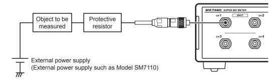
When using Model SM7110 or SM7120 as an external power supply, wire the system as follows: Connect the shorting plug to the GUARD terminal and the GROUND terminal. Connect an object to be measured to the OUTPUT terminal of Model SM7110/SM7120. Connect the GUARD terminal of Model SM7110/SM7120 and the COM terminal of Model SM7420 with each other.
