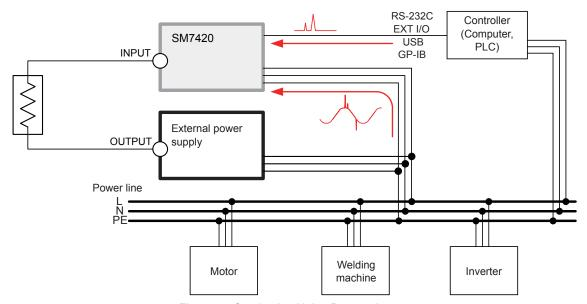
Figure 5 Conductive Noise Penetration
