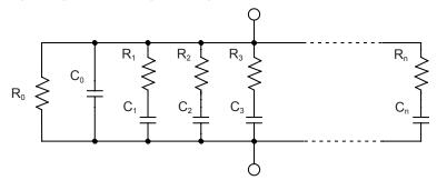
Figure 1 Equivalent Circuit of the Insulator
