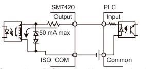
Connection to PLC input (positive common input)
