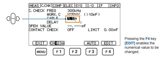
If using an accessory or an optional cable, press the **F4** key **[EDIT]** to specify its length. If the cable is modified or extended, it is recommended to press the **F3** key **[AUTO]**. Pressing the **F3** key **[AUTO]** executes the cable length correction once. If you change the cables, press the **F3** key **[AUTO]** to execute the cable length correction again.
