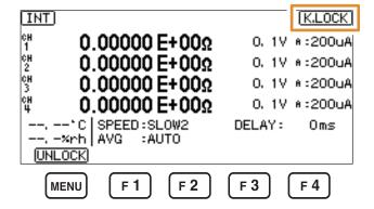
To unlock the key lock: hold the MENU key [UNLOCK] for more than 1 second.
