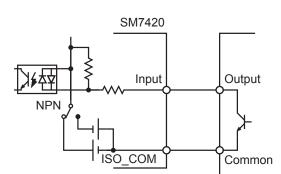
Connection to PLC output (NPN output)
