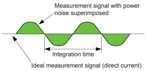
Figure 4 Noise caused by the commercial power
