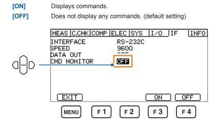
The communication monitor is displayed on the measurement screen when communication starts.
