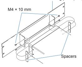
2 Install the spacers on both sides of the instrument, secure the rack mounting plate with the M4 × 10 screws.
