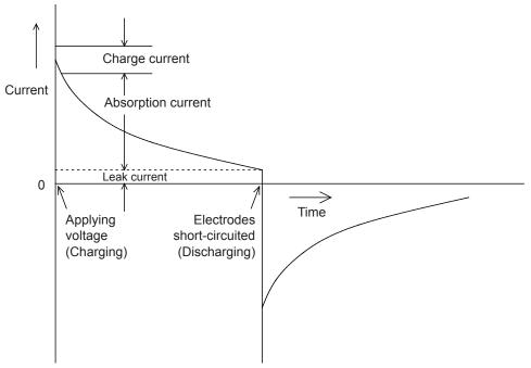
Figure 2 Dielectric Absorption
