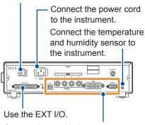
Communicate with the computer through USB, RS-232C, or GP-IB.
