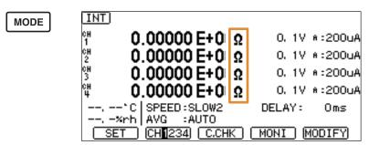
The instrument displays values that include the input resistance of 1 k $\Omega$  (±10%).
