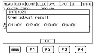
A short-circuit between the INPUT and OUTPUT terminals will cause the fixture capacitance open correction to fail, displaying a result "NG." Check a short-circuit between the terminals.
