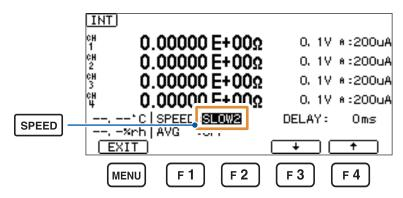
The measurement speed changes every time the F3 key [ $\downarrow$ ] is pressed in the following order: FAST, FAST2, MED, SLOW, and SLOW2.
