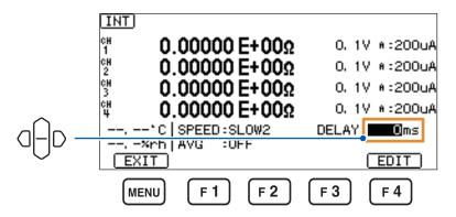
Pressing the **F4** key **[EDIT]** enables the numerical value to be changed in increments of 1 ms.
