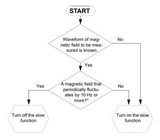
\*: When measuring a magnetic field that periodically fluctuates by 10 Hz or more, turn off the slow function.
