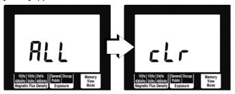
After this it displays the model number and estimated remaining battery life, and is restarted using the factory default settings.
