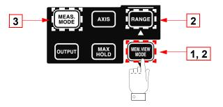
1. Press to open the screen with the saved measurement data.
