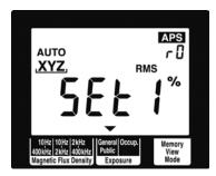
After this follow the procedures 2. (P.48) described in 3.4.3 "Measurement Procedure" to perform an exposure level (General Public) measurement.
