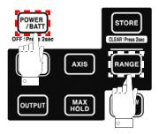
When the power is off, hold down and press POWER This deletes all saved measurement data.
