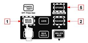
Press MEAS. to open the exposure level (Occup.) mode screen.
