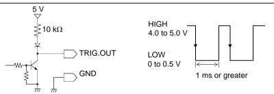
When triggering is not otherwise used, a trigger signal is output during measurement.
