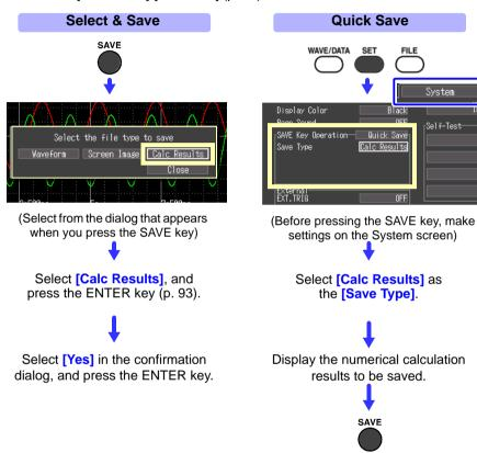
By specifying a particular time span for numerical calculation, only the results for that time span are saved.
