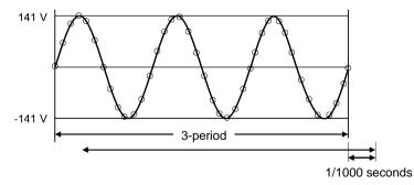
The 50 Hz or 60 Hz waveform is sampled for 200  $\mu$ s, and 1 RMS data point is calculated using data for 3 periods. Thereafter, RMS data is calculated at a 1/1,000 sec. interval.
