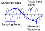
Aliasing occurs when the sampling period is longer than half of the input signal period.
