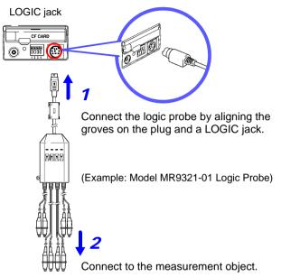
When a logic probe is not connected, the corresponding logic waveform appears at HIGH level on the waveform screen.
