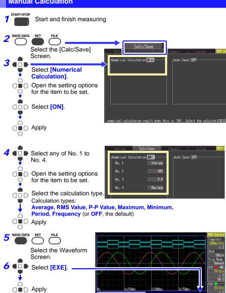
Analyze (p. 63) The results of numerical calculations are displayed on the Waveform screen. If needed, you can change calculation types and recalculate.
