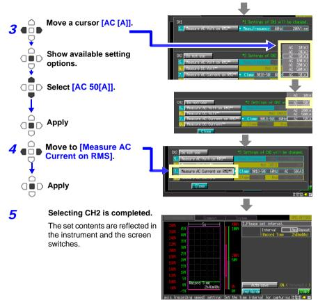
Configure the following settings after completing the content selection of CH1 and CH2.
