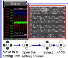
Select the timebase (horizontal axis), voltage range (vertical axis) and input channels.
