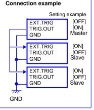
9.4 Synchronous Measurements with Multiple Instruments
