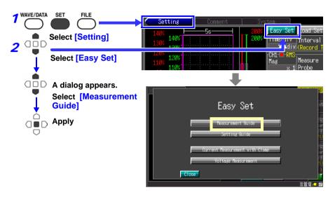
Configure the CH1 settings to measure AC voltage
