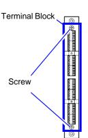
The terminal block can be detached from the Model 8958 16-Ch Scanner Unit.
