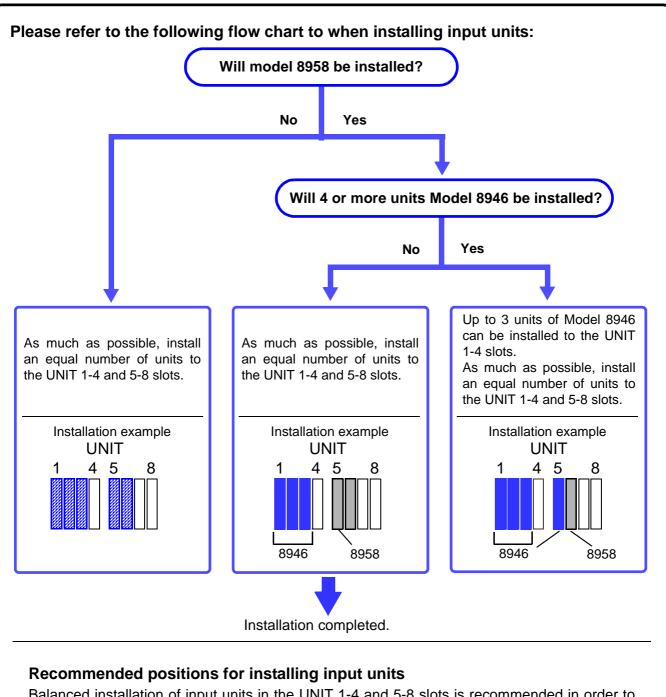
Balanced installation of input units in the UNIT 1-4 and 5-8 slots is recommended in order to effectively utilize the internal memory of Model 8861-50/8861-51.
