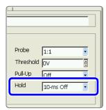
During measurement, the measured frequency value can be retained by the Hold function until the frequency of the next cycle has been determined. Also, if the value is not retained and the next value cannot be determined within a specified period, one half of the last measured value can be displayed.
