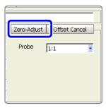
The input module can apply an internal offset to set the reference potential of the instrument to zero volts.
