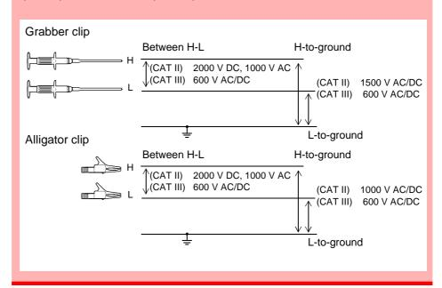
When using an input module (BNC jack) other than the Model 8940 F/V Unit
