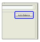
Auto-balance sets the reference output level of a transducer to the specified zero position.
