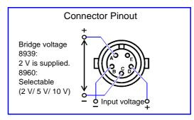
The grounds of the instrument and the Connector Shell of the 8960 are not isolated.
