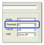
Sets threshold value. Measures when the waveform crosses a preset threshold. Setting Item: [Threshold]
