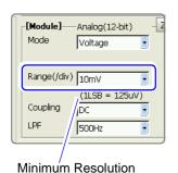
Select the appropriate measurement range. The setting value is the units per division on the vertical axis.
