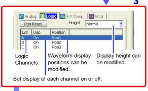
Use the **CURSOR** keys to move to a logic channel to be displayed, and press the F keys to select the setting contents for each item.
