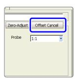
The input value can be forced to display as zero volts. Input signal bias, such as sensor emf, can be adjusted to display as zero volts. This function applies to voltage and current measurement.
