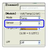
Set to match the type of thermocouple being used.
