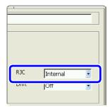
When connecting a thermocouple directly to the input module, select [Internal]. Reference junction compensation is performed within the input module. When connecting through a reference junction device (e.g., a 0°C control tank), select [External].
