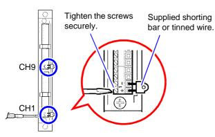
1 Short the + and – terminals of channels 1 and 9 on the Model 8958 16-Ch Scanner Unit to be adjusted.
