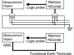
Connect the measurement object's ground to the GND terminal of this instrument. (Always obtain power from the same mains circuit.)
