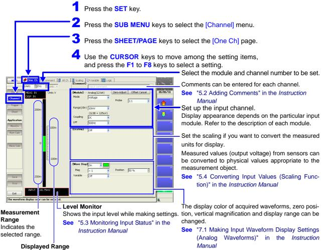
Indicates the range displayed on the screen. To change the display position or range, change the waveform display settings.
