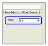
Probe attenuation can be selected when measuring using a connection cable, differential probe or attenuating probe. (Only for voltage measurement)
