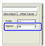
Noise can be removed by applying additional averaging to the measurement data within the input module.
