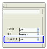
A broken thermocouple wire can be detected during temperature measurement. Normally when a thermocouple wire breaks, measured values exhibit random instability.
