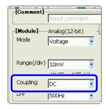
Select the coupling method for input signals
