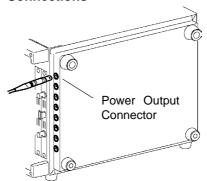
Connect the power cables from the probes to the output connectors of the Model 9687 Probe Power Unit.
