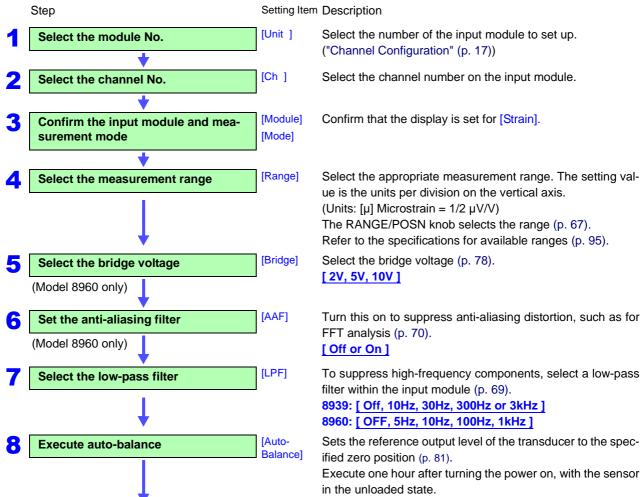
To suppress high-frequency components, select a low-pass
