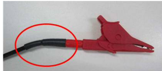
After the repair with heat shrink tube
