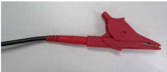
Before the repair (no heat shrink tube)
