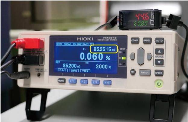
Fig. 6 Resistance value with temperature correction
