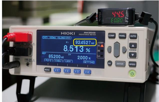
Fig. 7 Resistance value without temperature correction
