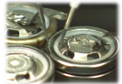
The probing repeatability is extremely important for measuring ultra-low resistance with high-accuracy. Excellent probing precision and repeatability accuracy keeps exactly same measurement point, ensuring high stability measurement. Keeps stable 4-terminal measurement method even though extreme narrow space like external case edge of negative electrode of cylinder-shape cell.
