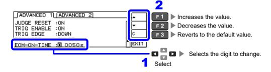
The output time cannot be set unless the output method is set to pulse.
