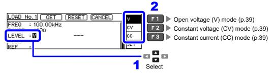
Enter the compensation signal level voltage or current value.
