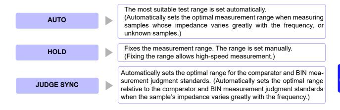
NOTE The ranges are all defined in terms of impedance. Therefore, for a parameter other than impedance, the value is obtained by calculating from the measured values of |Z| and  $\theta$ . See "Appendix1 Measurement Parameters and Calculation formula"(p. A1)
