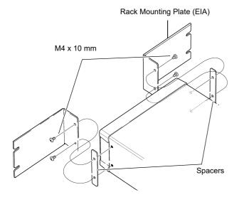
Installing the spacers on both sides of the instrument, affix the Rack Mounting Plate with the M4 x 10 mm screws.
