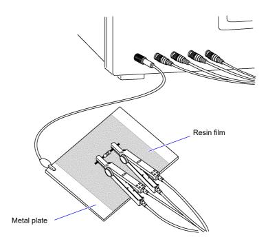
When measuring components on a metal plate, use, for example, resin film as insulation to ensure terminals and the like are not short-circuited.
