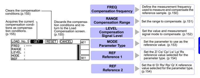
The compensation coefficient is computed from the reference values of Z and  $\theta$  obtained from the set values and the actual data acquired from the reference sample at each of the compensation frequencies.
