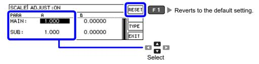
Enter a value for compensation coefficient A with the tenkey and accept it with the **ENTER** key. **10KEY**
