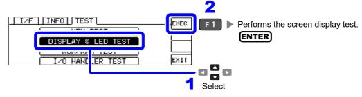
Each time you press **ENTER**, the screen and the LEDs on the front of the instrument will cycle on and off in the following order:
