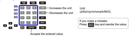
When entering a value for compensation coefficient A, the [x10²] [+10²] keys are disabled.
