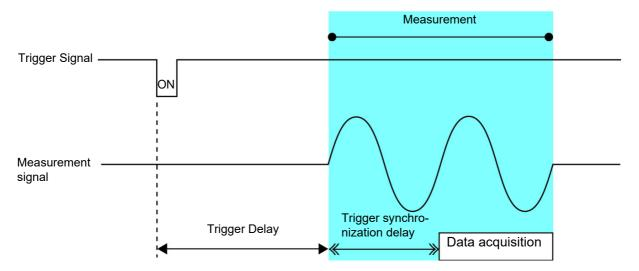
When the range synchronization function has been set, the range settings at which the trigger delay and trigger synchronous output function are enabled vary with the parameter settings.
