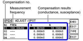
You can check the conductance and susceptance at compensation points with
