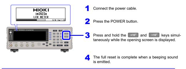
If the instrument still does not operate normally after the full reset, it needs to be repaired. Contact your authorized Hioki distributor or reseller.
