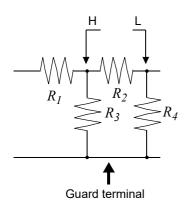
If as shown in the next figure a guard terminal is used, the current flowing through the resistors  $R_3$  (not flowing through  $R_4$ ) is absorbed by this guard terminal, so that the resistance value for the resistor  $R_2$  is accurately measured.
