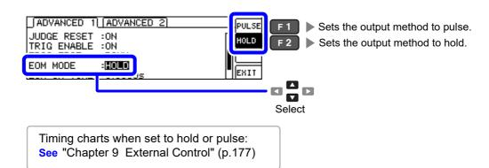
Select [EOM-ON-TIME] and set the EOM output time to use with pulse EOM mode.
