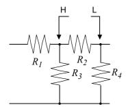
Referring to the following figure, when measuring a resistance value for the resistor  $R_2$ , even if the tips of the two probes are contacted against the ends of the resistor  $R_2$ , considering the sum of the current flowing through the resistor  $R_2$  and the current flowing through the resistors  $R_3$  and  $R_4$ , what is obtained is the resistance value for the parallel combination:
