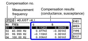
When compensation completes normally, the conductance and susceptance will be displayed. Compensation is supported for impedance values of 1 k $\Omega$  or greater.
