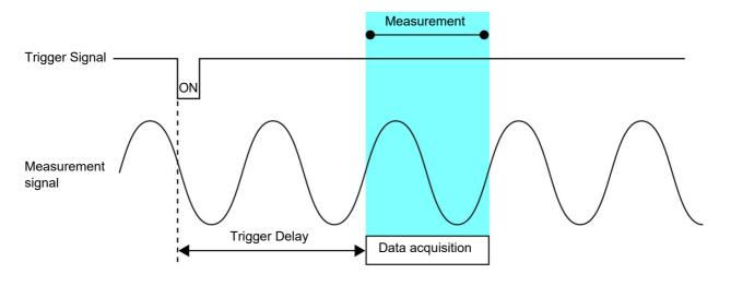
Trigger delay: ON; Trigger synchronous output: ON
