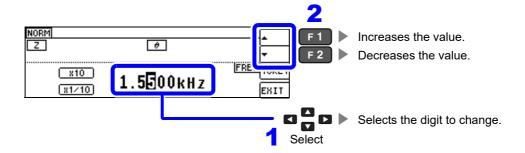
NOTE The digits in the measurement frequency can also be changed using the **\times** keys.
