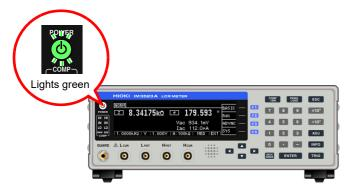
To ensure that measurements fulfill the degree of accuracy described in the specifications, allow the instrument to warm up for at least 60 minutes after it is turned on.
