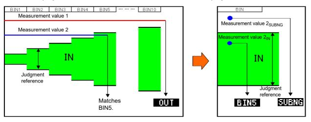
In BIN judgment, a judgment is made based on the main measurement value first, and then the result of a judgment using the sub measurement value is output. In the above example, is displayed since main measurement value 1 did not fulfill any of the set judgment standards. Main measurement value 2 was the first to fulfill the standard, and **SUBJET** is displayed since the judgment standard set for BIN5 was fulfilled.
