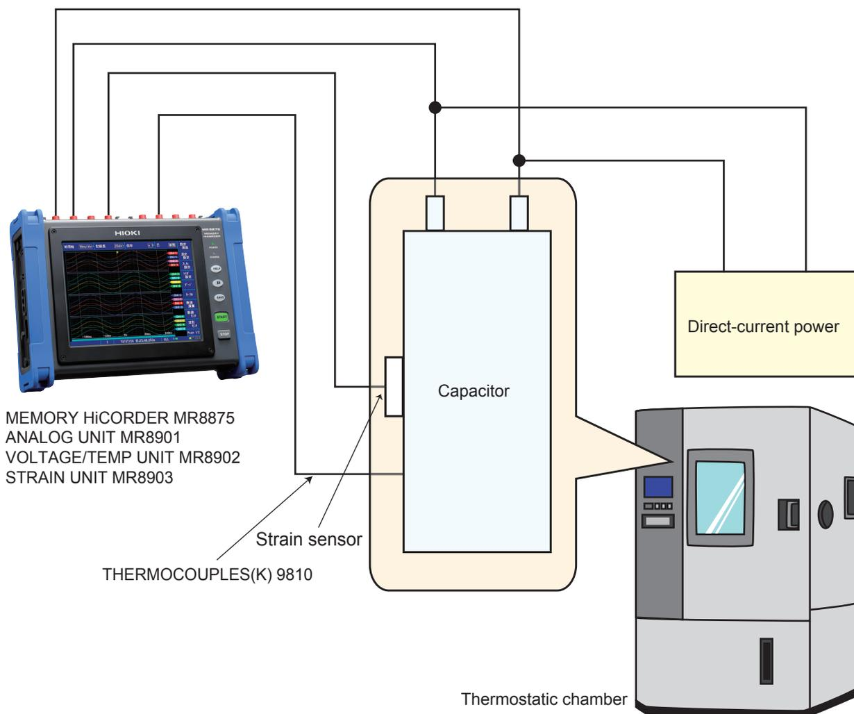
Thanks to its ability to operate on battery power and its compact, lightweight design, the MR8875 can boost measurement efficiency in the field.
