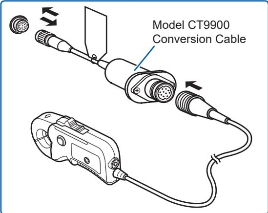
When Model CT9900 Conversion Cable is used, the instrument recognizes Model CT6846 or CT6865 (1000 A rating) as a 500-A AC/DC sensor. Set the conversion ratio to 2.00.
