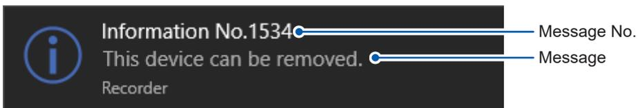
Some of the warning and information messages disappear in a few seconds. Check the details while the screen is displaying the message.
