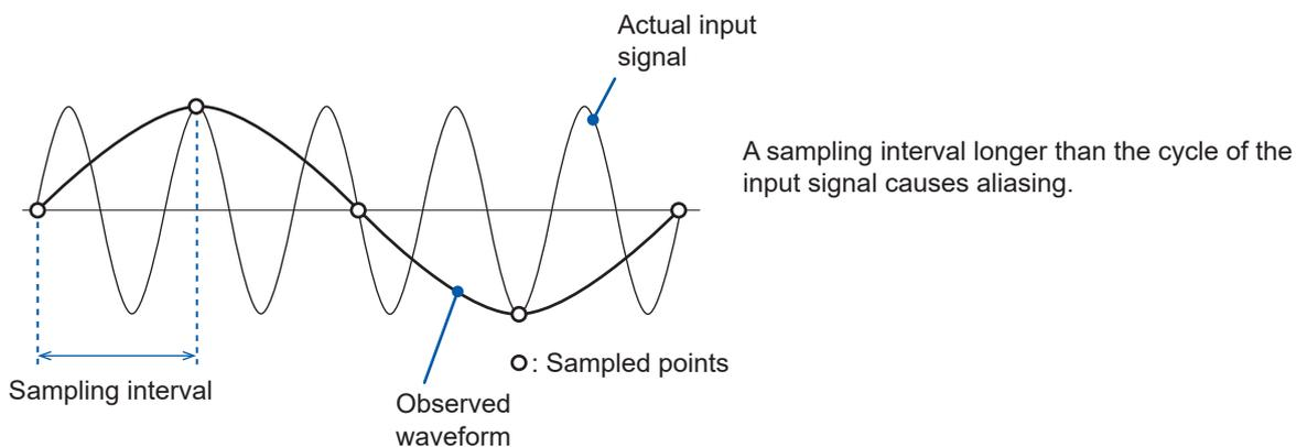
To plot a sign wave that allows you to observe the peaks without any aliasing, the instrument needs to sample the waveform at a minimum of 25 points per cycle.
