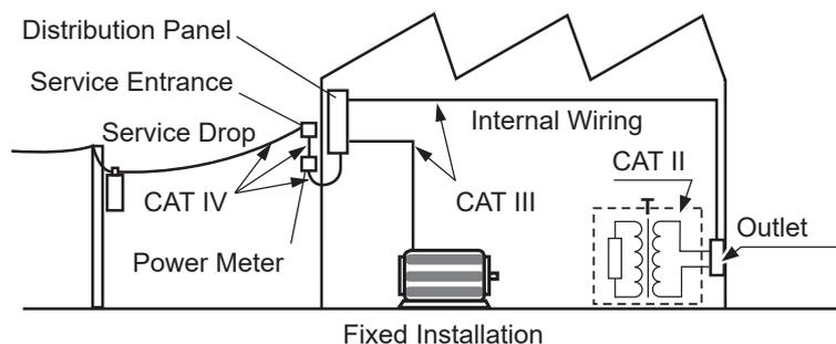
The applicable measurement category is determined based on the module being used. Refer to “Handling the instrument and modules” (p. 10).
