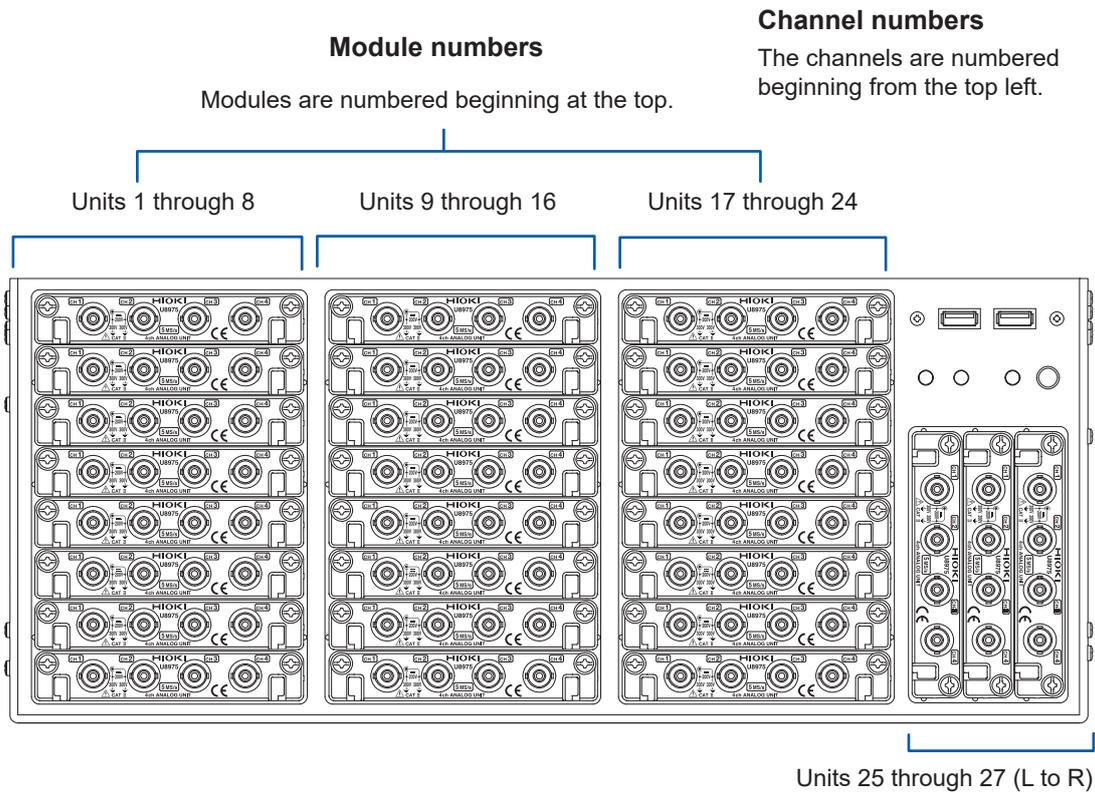
Model 8973 Logic Unit can be installed in slots to which Unit 25, 26, or 27 is assigned only.
