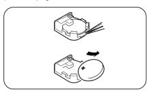
Insert tweezers or other similar pointed tool between the battery and the battery holder. Raise the battery to remove.
