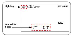
4. To start the step voltage test, hold down the key for more than one second.
