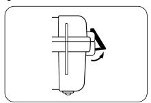
While raising the entire latch, place a finger on the top of the latch and pull it out.
