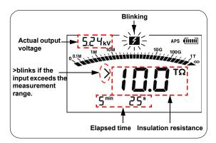
If > blinks, the input value is out of measurement range. Example: > 10.0 T $\Omega$  means "larger than 10.0 T $\Omega$ ."
