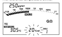
5. Adjust the reference temperature using the key.
