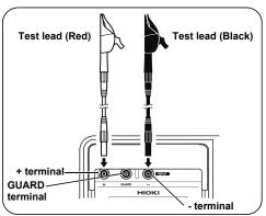
4. Clip the ends of the test leads to the circuit to be tested. When the voltage exceeds 50 V, the mark and key mark amp blink.
