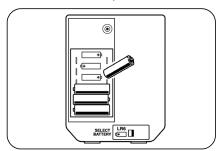
Turn the battery selector switch to LR6. When the power is turned on, "Lr6" appears on the top left of the screen.
