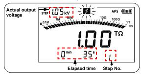
The test voltage rises at regular intervals and the test stops automatically.
