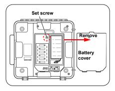
Place six LR6 Alkaline batteries or six HR6 Nickel-metal hydride batteries into the battery compartment. (Replace all six at the same time)
