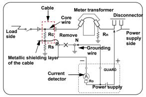
Rc: Insulation resistance of the insulating material of the high-voltage cable (Between core and metallic shielding layer)
