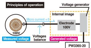
Inside the PW9020 is an electrode (a metal plate). When there is a potential difference between this electrode and the measured line, a minute current flows as a result. By detecting this minute current and generating a voltage such that the current declines to zero, it is possible to accurately measure the voltage without being affected by the outer diameter of the measured cable or its insulation.
