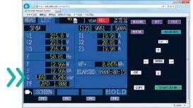
Display the power logger's screen and make adjustments virtually by clicking the buttons and entering new information.
