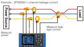
With the ability to calculate and process data every 200ms, you can do simple checks of intermittent leakage current. Choose from average, maximum and/or minimum value of the measured interval.
