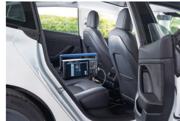
Analyzing power conversion efficiency in driving tests of finished vehicles
