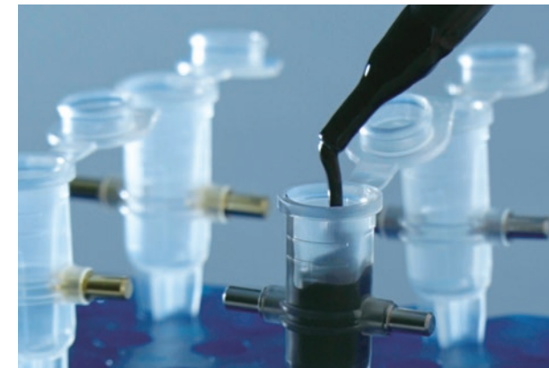
Evaluating the performance of slurry, a raw material for batteries
