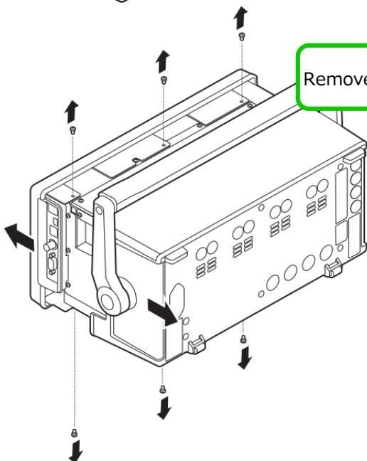
Remove the six screws securing the front
