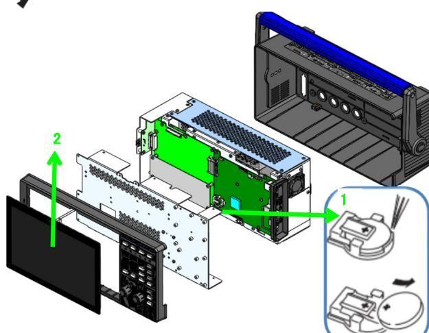
Insert the tweezers between the battery holder on the internal printed circuit board and battery to remove the battery.
