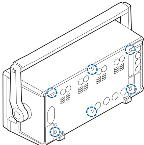
Remove the six screws securing the rear
