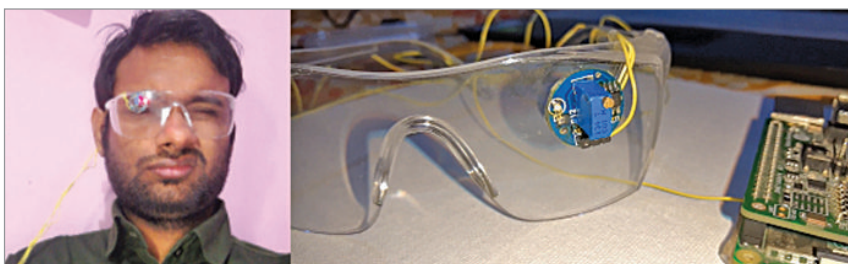
Fig. 2: Author testing the blink sensor
