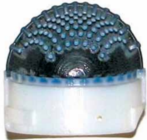
Robotic finger tip makes human-like ‘nerve’ signals (Credit: https://www.electronicweekky.com )
