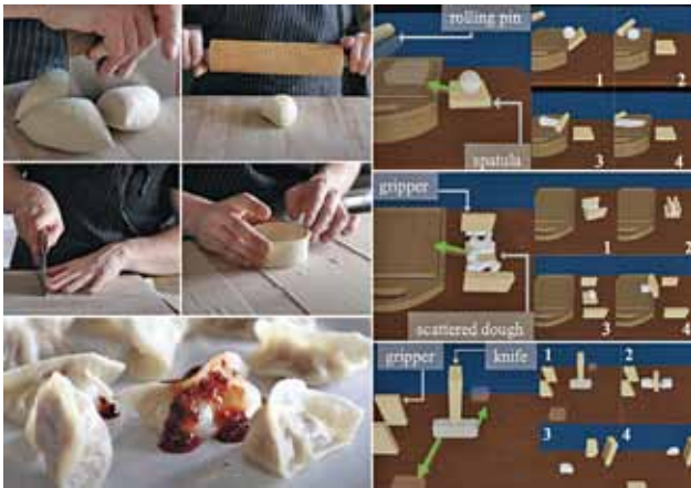
Researchers from MIT and elsewhere have created a framework that could enable a robot to effectively complete complex manipulation tasks with deformable objects, like dough or cloth, that require many tools and take a long time to complete (Credit: https://news.mit.edu )
