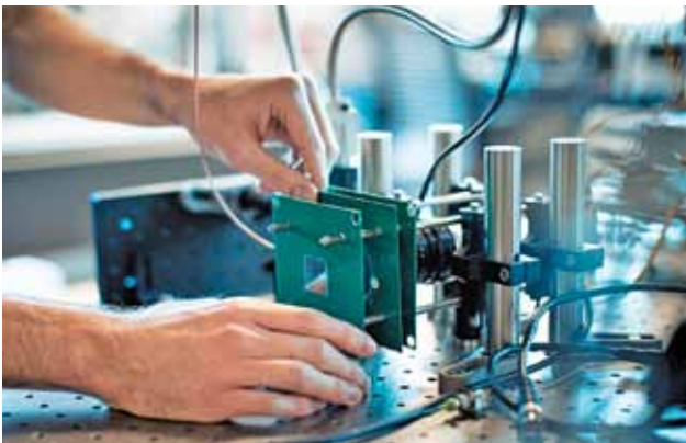
The lab-based prototype lidar system that the research team built, which successfully captured megapixel-resolution depth maps using a commercially available digital camera (Credit: https://news.stanford.edu )
