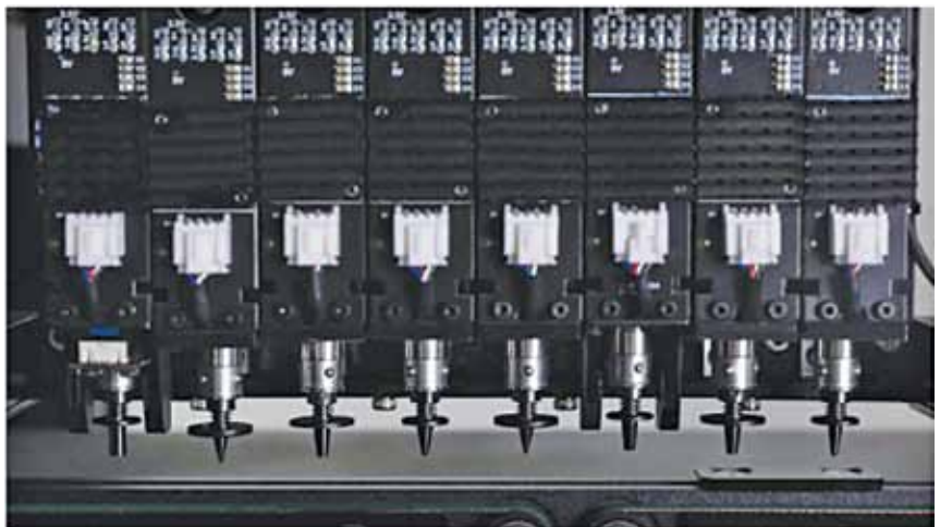
Eight synchronised nozzle heads of Neoden 8
