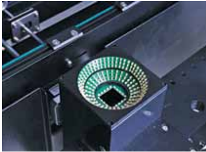
Vision system inside Neoden 8 PnP machine (Credit: https://neodenusa.com )
