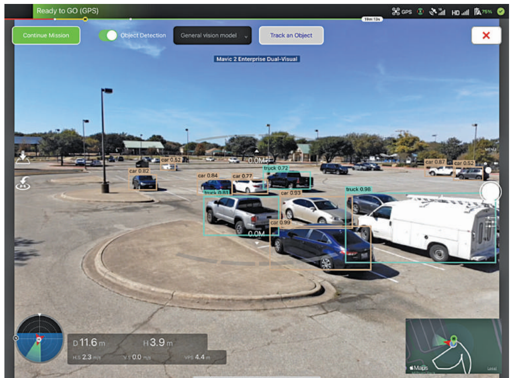
Drone Skygrid, an airspace management system built on AI and blockchain, uses computer vision for near real-time object detection through a drone's live video stream (Credit: Skygrid)
