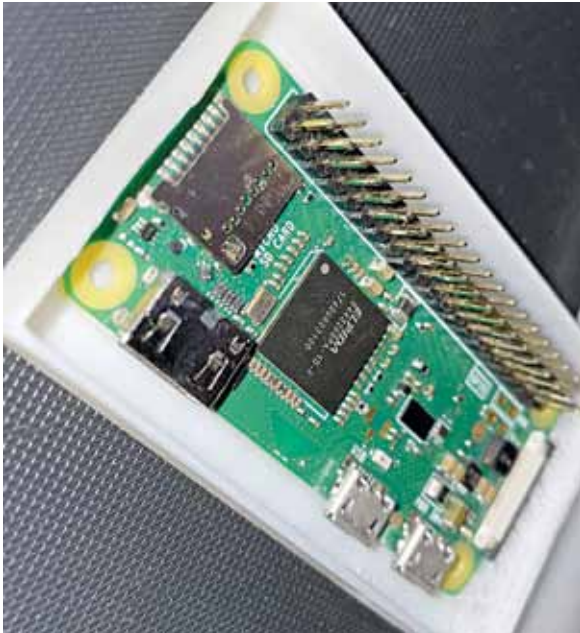
Fig. 14: E-ink header-to-header pins on Raspberry Pi
