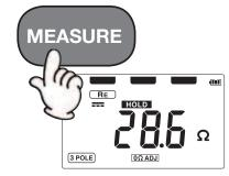
The FT6031-03 automatically checks the ground potential, checks the auxiliary grounding electrode, and measures the grounding resistance. The instrument also selects the optimal range for the grounding resistance, eliminating the need to switch ranges and enabling efficient measurement.
