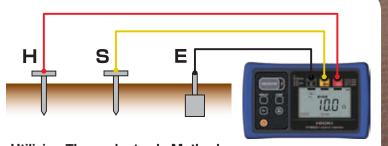
**Utilizing Three-electrode Method**
