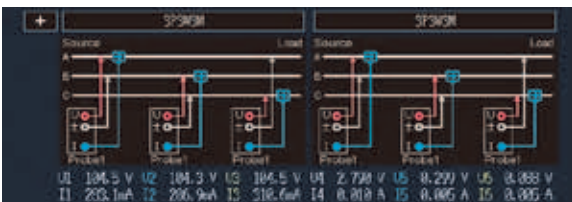
Wiring confirmation function, to avoid wiring mistakes
