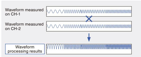
Simultaneously make up to 16 waveform calculations by combining the four arithmetic operations and 11 types of calculations
