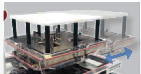
Long-stroke design can be used with characteristics evaluation techniques that require large position shifts, for example the magnetic resonance method.
