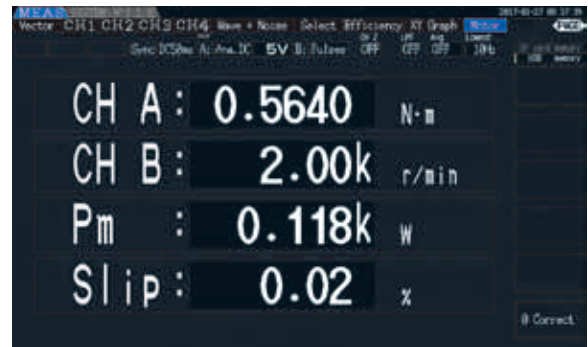
Motor analysis screen (Torque, rotation rate, motor power, slip) For CH B, enter the Z-phase pulse of the encoder to measure electric angle, and enter the B-phase pulse to measure rotation direction.
