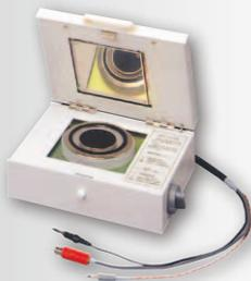
Sample of 100mm square by up to 8mm in thickness is measurable. The main electrode dia. is 50mm and inner & outer dia. of ring electrode are 70mm & 80mm respectively. Measurement voltage becomes "OFF" while the lid is open to ensure safety. A selector switch allows selection of voltage or surface resistivity.
