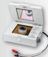
Sample of 40~100mm square by up to 8mm in thickness is measurable. The main electrode dia. is 19.6mm and inner & outer dia. of ring electrode are 24.1mm & 28.8mm respectively. Measurement voltage becomes "OFF" while the lid is open to ensure safety. The fundamental specifications are the same as SME-8310.
