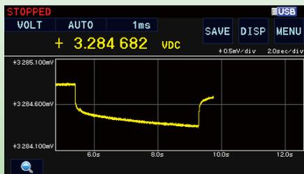
DC-IR measurement waveform for a battery
