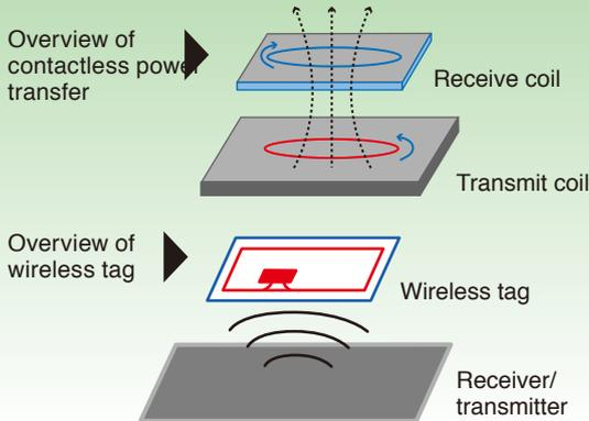
Contactless power transfer technology, which lets you charge mobile phones and consumer electronics like phones, electric toothbrushes, and electric shavers simply by placing them on a stand, is becoming increasingly common. Research into the commercialization of high-capacity contactless power transfer as a technology for charging electric vehicles and plug-in hybrid vehicles is progressing at a rapid pace.
