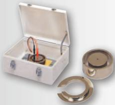
This is an electrode for plate sample for use together with SME-8350 shield box. This electrode enables extremely easy measurement of surface resistivity and volume of sample with coarse surface such as carpets, etc. The main electrode dia. is 50mm, and the ring electrode inner-dia. and outer-dia. are 70mm and 80mm respectively.
