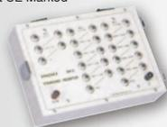
This is a resistor box for calibration of the super megohmmeters. Max. voltage is 1,000 V DC and resistor value covers from 10 M $\Omega$  to 10,000 M $\Omega$  in 24 points.
