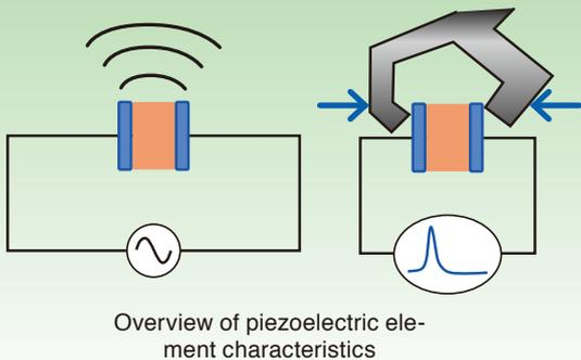
Piezoelectric elements convert electric signals to mechanical movement and vice versa. When an electrical signal is applied externally, the element's shape changes, allowing it to be used in buzzers and other sound-producing components. Another example is its application in pressure and inclination sensors, whereby an electrical signal in response to changes in the element's shape is output.
