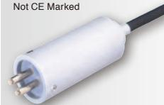
Electrode for surface resistance of curved samples such as resin and rubber processed goods, TV cathode tubes or small samples. Surface resistance can be measured by pressing the rubber tips at the tip onto the sample. Measure electrodes up to  $10^{11} \Omega$  at 10mm intervals or greater.
