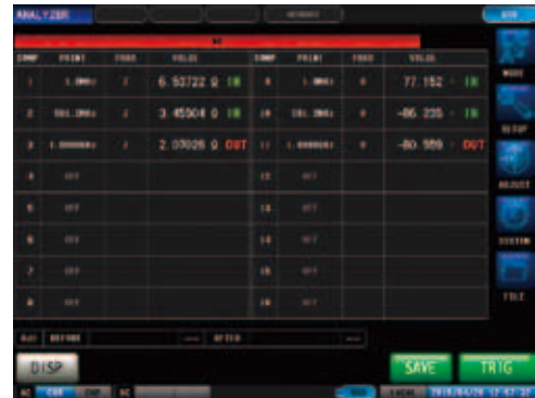
For multiple-frequency pass/fail judgments: [Analyzer mode : Spot judgment]
