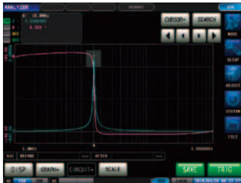
For pass/fail judgments based on frequency characteristics: [Analyzer mode : Peak judgment]
