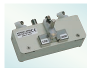
SMD TEST FIXTURE 9699 Direct connection type, For measuring SMDs with electrodes on the bottom; DC to 120 MHz, test sample dimensions: 1.0 mm (0.04 in) to 4.0 mm (0.16 in) wide, max. 1.5 mm (0.06 in) high
