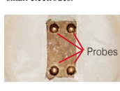
SMD TEST FIXTURE 9699 Direct connection type, For measuring SMDs with electrodes on the bottom; DC to 120 MHz, test sample dimensions: 1.0 mm (0.04 in) to 4.0 mm (0.16 in) wide, max. 1.5 mm (0.06 in) high
