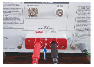
**4** Slide the stopper plate downward until it comes in contact with the screws and locks the connectors in place.
