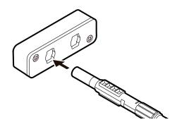
2 Insert the unterminated lead cable connector all the way inside.
