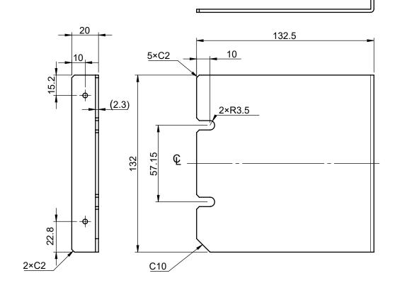
Unit: mm, Material: SECC (electro-galvanized steel sheet), Thickness: 2.3
