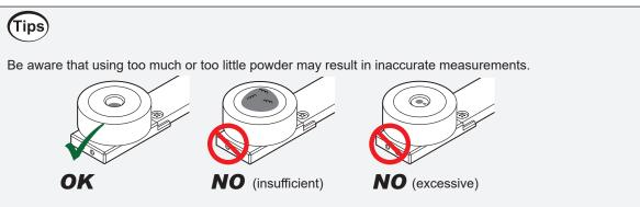
5 Hold the handle of the lower electrode and tap it on a flat surface to remove air from the powder.
