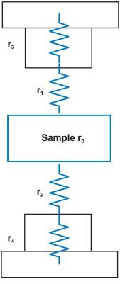
Measured value  $R = r_0 + r_1 + r_2 + r_3 + r_4$
