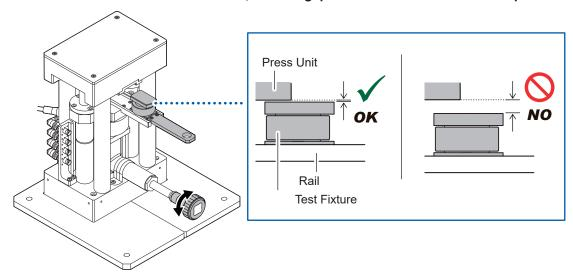
**4** Securely insert the Test Fixture deeply into the rail.
