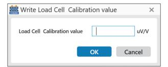
2 Enter the rated output value from the Test Data Sheet of the load cell included with the Press Unit into the Load Cell Calibration value box, illustrated in step 1.
