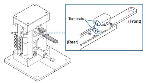
2 Attach the quick spinner to the hydraulic jack of the Press Unit.
