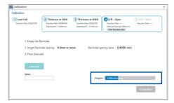
When the open compensation is successfully completed, the short compensation starts.
