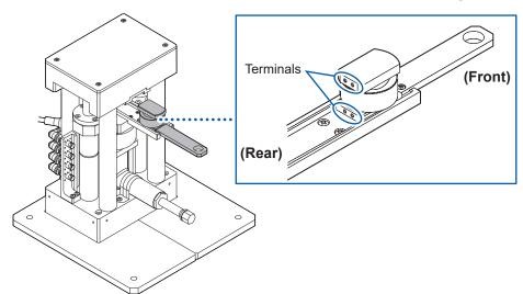
Attach the quick spinner to the hydraulic jack of the Press Unit.
