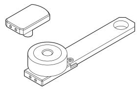
4 Place the powder with the mass specified in the [Material Info] field (p.80) into the recess of the Test Fixture.
