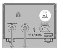
Connect the USB cable to the USB connector of the Sensor Unit.
