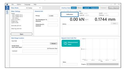
6 With no load applied to the Test Fixture, click [Execute].
