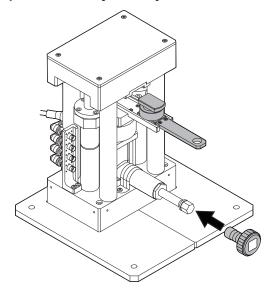
3 Turn the quick spinner to adjust the height of the Test Fixture so that its upper electrode does not contact the Press Unit, and the gap between them is as small as possible.
