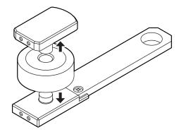
2 Position the powder release pin and the guide plate on the die.
