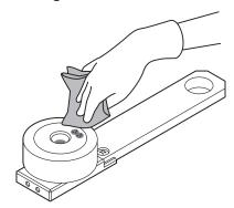
Position the upper electrode of the Test Fixture onto the die, and rotate the upper electrode several times to flatten the powder in the recess.
