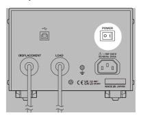
**2** Connect the accompanying power cord to the power inlet of the instrument.
