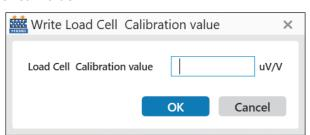
Entering the Load-Cell Calibration Value to the SA2653 Measurement Software
