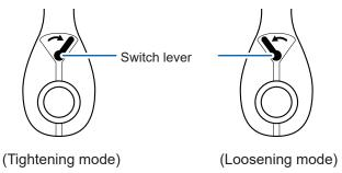
2 Use the ratchet handle in tightening mode to turn the hydraulic jack screw clockwise and apply a load to the powder filled in the Test Fixture.
