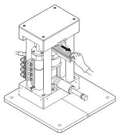
2 Attach the quick spinner to the hydraulic jack of the Press Unit.
