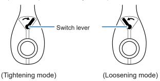
Use the ratchet handle in loosening mode to turn the hydraulic jack screw counterclockwise and zero the load to the powder filled in the Test Fixture.
