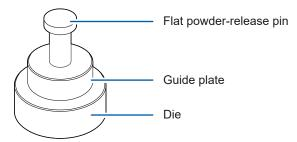
3 Position the die, the guide plate, the powder release pin, and the tray in the SA9005 Mold Release Unit.
