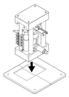
Insert the bases through the pass box into the glove box.
