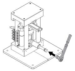
Using the switch lever of the ratchet handle can switch between two ratchet handle modes: tightening mode (clockwise) and loosening mode (counterclockwise).
