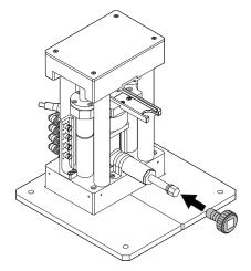
3 Turn the quick spinner to minimize the protrusion of the hydraulic jack screw.
