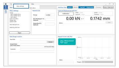
3 Select the options for measured-value display formats used in the SA2653 Measurement Software.
