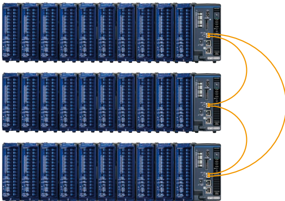
Example of synchronized measurement with 3 loggers
