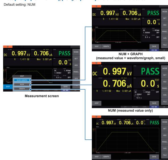
GRAPH (measured value, small + waveform/graph, large)
