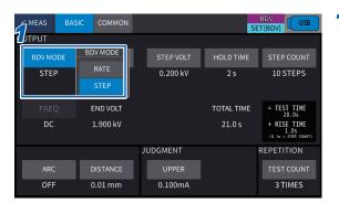
On the setting screen, press [BASIC] > [BDV MODE] to set the test method to [RATE].
