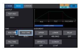
Press [BASIC] > [TEST TIME] on the setting screen.
