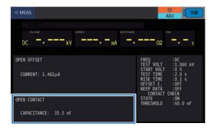
After the test finishes, the compensation value is acquired.
