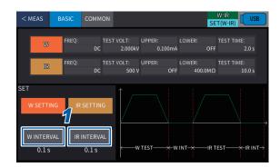
1 Press [BASIC] > [W INTERVAL] or [IR INTERVAL] on the setting screen.
