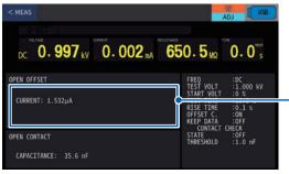
When the test ends, the current compensation values are acquired.
