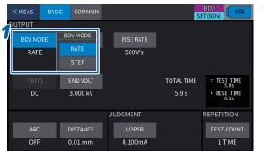
Press [BASIC] > [BDV MODE] to set the test method to [STEP].
