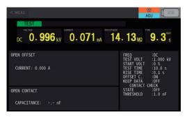
Press [ADJ] on the measurement screen and start the test on the compensation execution screen.
