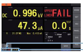
On the measurement screen, a contact check is executed at the end of the test.
