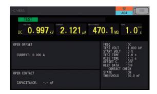
Press [ADJ] on the measurement screen to start a test on the compensation execution screen.
