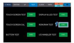
1 Press [SYS] > [TEST] > [EXEC] of [ROM/RAM TEST] on the measurement screen.
