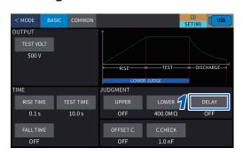
1 Press [BASIC] > [DELAY] on the setting screen.
