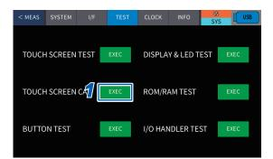
1 Press [SYS] > [TEST] > [EXEC] of [TOUCH SCREEN CAL] on the measurement screen.
