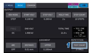
1 Press [BASIC] > [TEST COUNT] on the setting screen.
