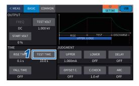
Press [BASIC] > [TEST TIME] on the setting screen.
