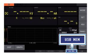
When the USB flash drive is properly recognized, the USB memory icon turns blue.
