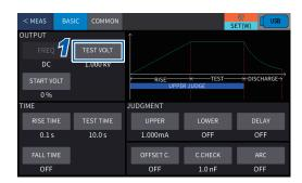
1 Press [BASIC] > [TEST VOLT] on the setting screen.
