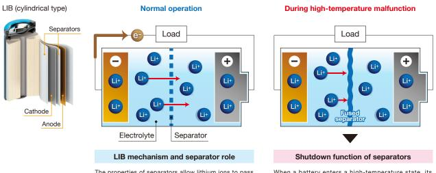
The properties of separators allow lithium ions to pass through them while maintaining electrical insulation. The entire assembly operates as a battery when lithium ions move through the electrolyte. When a battery enters a high-temperature state, its separators will fuse, closing off the holes in them and blocking the movement of lithium ions. As a result, the battery will stop operating to prevent a hazardous state.
