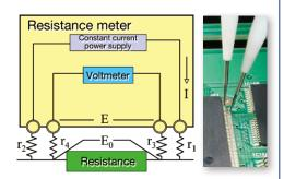
■ 4-terminal resistance measurement The connection resistance of probes is cancelled for accurate measurement of resistance between terminals. This measurement method is built-in for upper DMM models.
