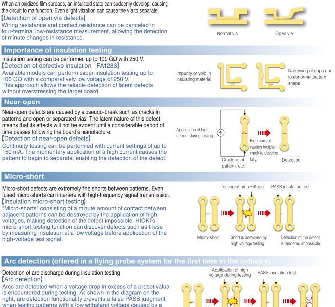
when testing patterns with a low withstand voltage caused by a tiny protuberance or other shape on one of the patterns, which is burned away when the arc occurs. When such a discharge is detected during testing, the location is judged to suffer from an arc defect, even if the insulation resistance value subsequently exceeds the reference value
