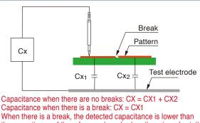
the capacitance of the reference board; when there is a short, the detected capacitance is higher than the reference board due to the additional capacitance of the other pattern.
