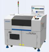
■ FLYING PROBE TESTER **FA1813** Testable board size 50×50 mm to 400×330 mm (max. 15.75×12.99 in)
