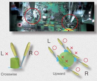
Probes are installed at an angle to allow probing of adjacent lands. At probing points near tall components, it is essential to check for interference between angled probes and components and to configure settings to avoid that eventuality.
