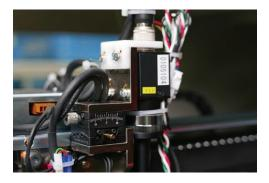
Unit is specially designed to minimize misalignment between the each alignment camera's optical axis and its probe's stroke.
