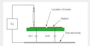
Capacitance value without break: Cx = Cx1 + Cx2Capacitance value with break: Cx = Cx1
