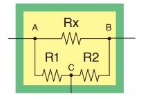
Guarding allows parallel elements to be isolated and measured individually.
