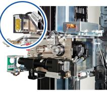
Laser board thickness compensation function
