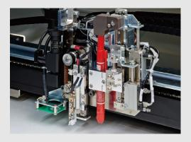
**DOT MARKING FUNCTION E4603** Dot marking using commercially available oil markers
