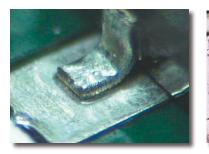
• Poor soldering Solder wicking is poor and the connection resistance has not decreased enough. This passes an operation (powered) test and therefore leads to unidentifiable malfunctions.
