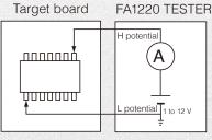
Current Test Block Diagram
