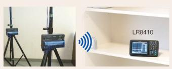
Data is sent wirelessly from measurement units to the LR8410.
