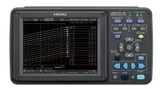
The communications range between the LR8410 and measurement units/wireless loggers is 30 m (line of sight). The communications range may be reduced if there are obstructions (such as walls or metallic shielding) between the devices.
