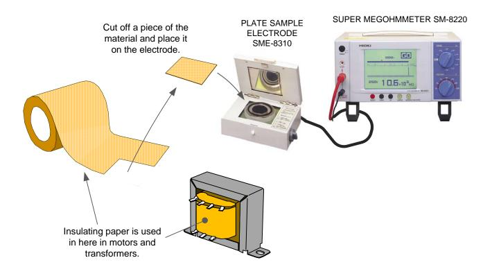
Insulating paper, which is inserted into transformers and motors, is manufactured by soaking paper in oil and then drying it. Excessive drying can cause the formation of cracks during processing, while inadequate drying can result in insulation defects. To ensure a consistent level of quality, the Super Megohmmeter SM-8220 can be used to manage the insulating state of the paper numerically.
