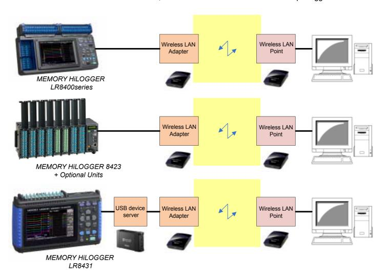
Use IO DATA model WN-AG300EA-S wireless access point and adapter set, and IO DATA model ETG-DSUS-HS USB device server.
