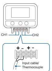
1 Loosen the terminal block screws. Insert the wires of the cable as shown in the figure and tighten the screws.
