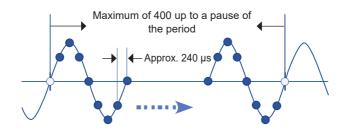
The value fluctuates significantly with an AC signal under 30 Hz.
