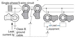
2. If any short-circuit is found, inspect from the power supply to the load using batch measurement (circuit clamped all at a time).
